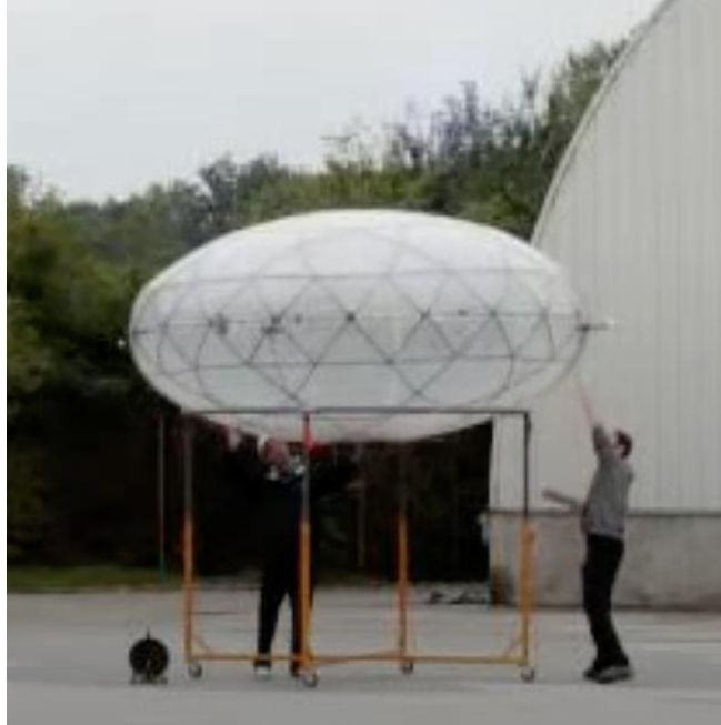
1SM airship recovered on a landing ring after a test flight. Source: Screenshot from Hipersfera video (Nov. 2010)
