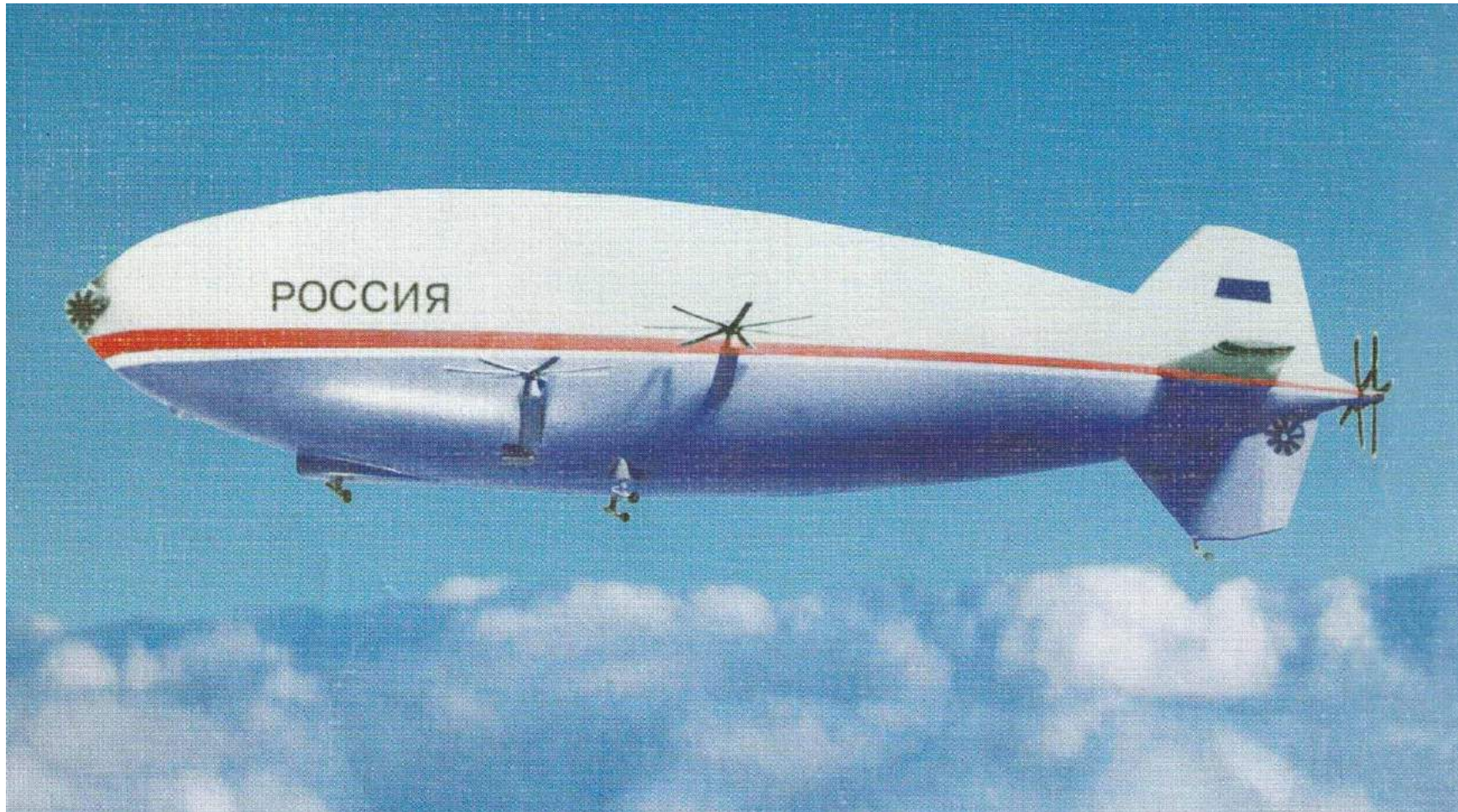
Rendering of an Aerolet 150 in flight. Note the tail-mounted coaxial propulsion propellers, the port-side vertical control rotor amidships (aft), the “lifting – lowering” rotor amidships (forward), and the lateral control propellers in the nose and tail fin. Source: Boyko (2001)
