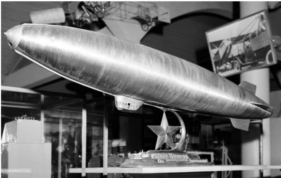
Model of an all-metal dirigible designed by Tsiolkovsky, on display at the Museum of the Yury Gagarin Order of the Red Banner and Order of Kutuzov Air Force Academy. Source: Runov/RIA Novosti
