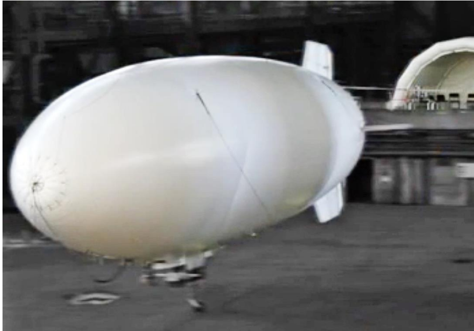
GA-22 inflation test. Source: Screenshot from Lindstrand Technologies video (2008)
