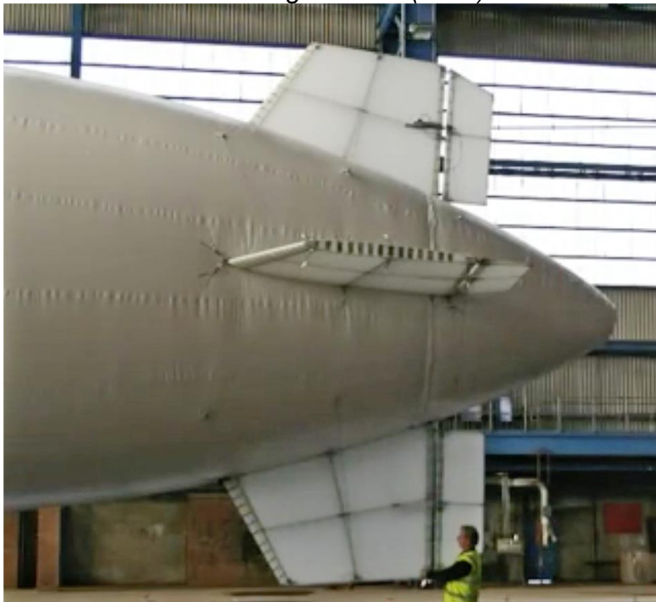
GA-22 tail fins attached for inflation test. Source: Screenshot from Lindstrand Technologies video (2008)
