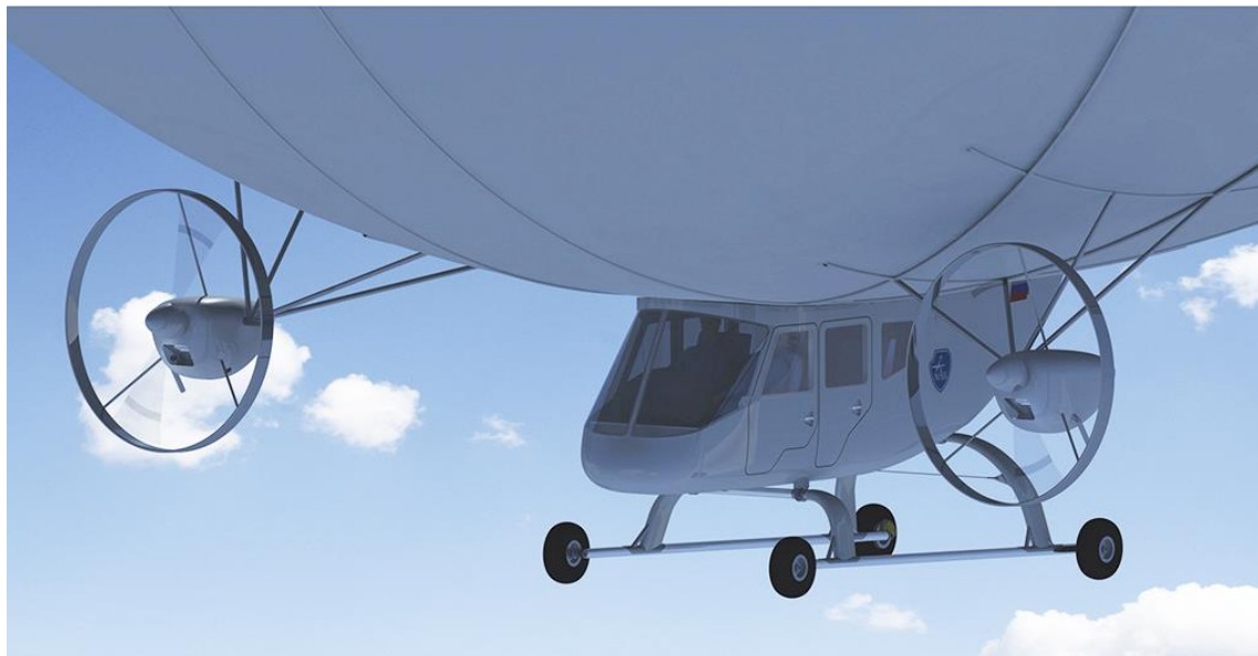
Closeup view of the four-passenger gondola and the two fixed Rotax engines supported from the gas envelope. Source, both graphics: OSKBES MAI
