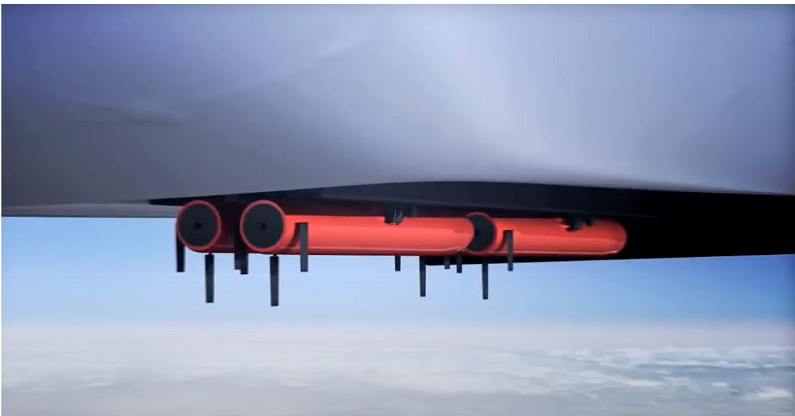
Tandem Gladius UAVs in Armatov weapons launcher. Source: Screenshot from MBDA video (2012)
