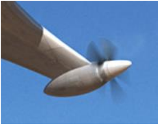
The two forward wings each carry a large podded tractor propeller.
