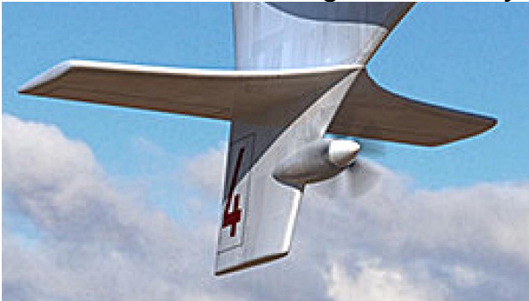
A third podded tractor propeller is mounted on the ventral tail.
