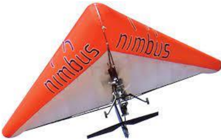
Nimbus Eos Xi viewed from below, highlighting the leading edge of the inflated delta wing.
