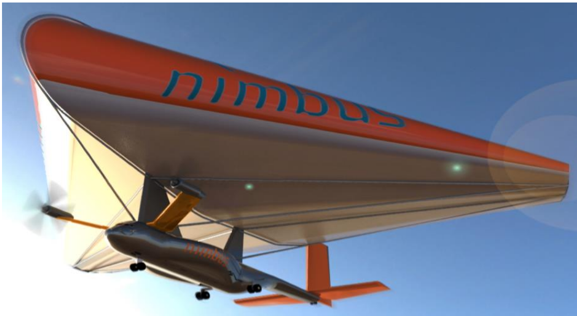
Rendering of a large Metaplano semi-buoyant aircraft in flight (general arrangement is representative of models T10 to T30) Source: Nimbus
