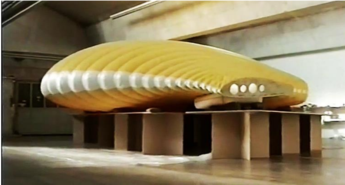
Stingray wing 1st inflation test on 17 Feb 1995. The tips of the wing are terminated with an endplate through which the spars will pass and to which wingtips will be attached later. Source: Prospective Concepts AG video (1995)
