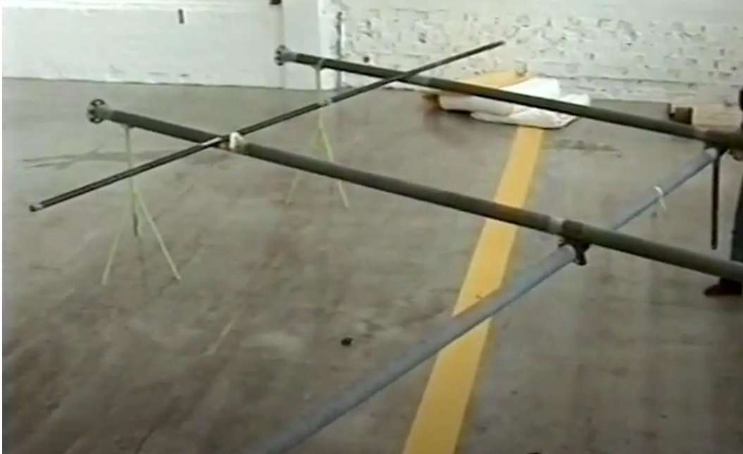
The aft end of the carbon fiber frame, from the aft wing spar (right side) to the attachment points for the tailplane assembly.
