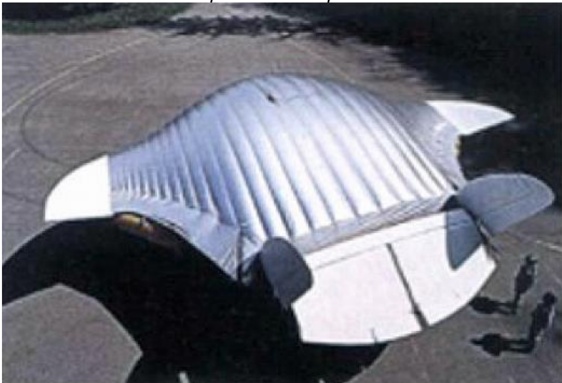
Stingray on the ground with elevators fully extended. Source: Prospective Concepts AG brochure
