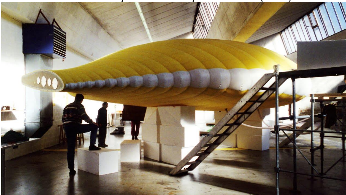
A later inflation test. Source: Screenshots from video, Stingray Part 2 (2020)
