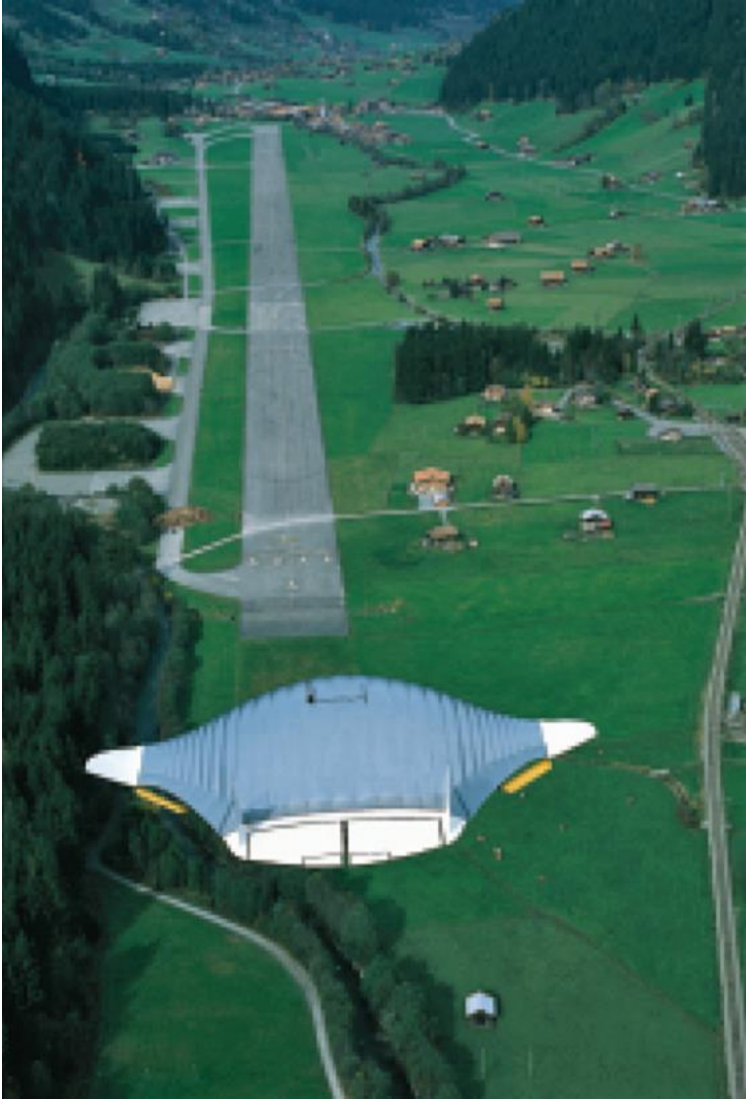
Stingray on landing approach at St. Stephan airfield. Note the yellow ailerons and the split elevator with trim tabs. Source: Prospective Concepts AG brochure
