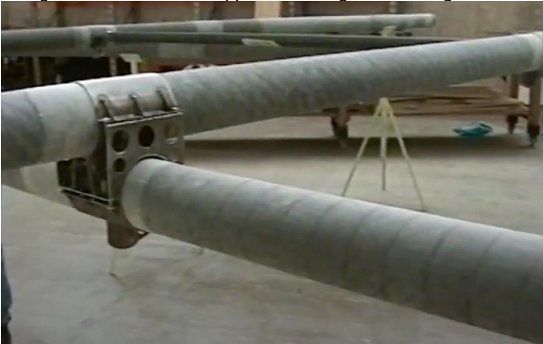
Closeup of mechanical joint for wing spar (foreground) and starboard longeron, with an attachment point for one vertical gondola support. Source, both photos: Screenshots from video, Stingray Part 2 (2020)
