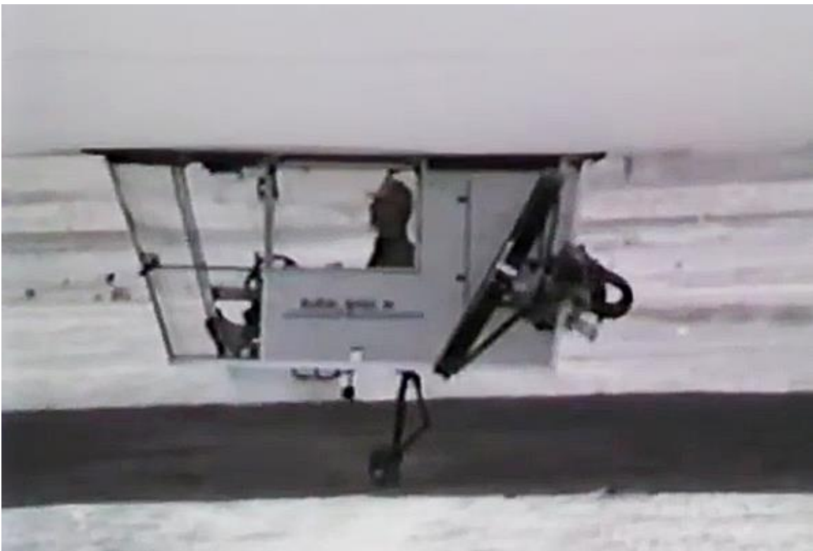
BA-2 gondola with propellers vectored partially up for a rolling takeoff. Source, both photos: Screenshots from Frank Rider video circa 1988
