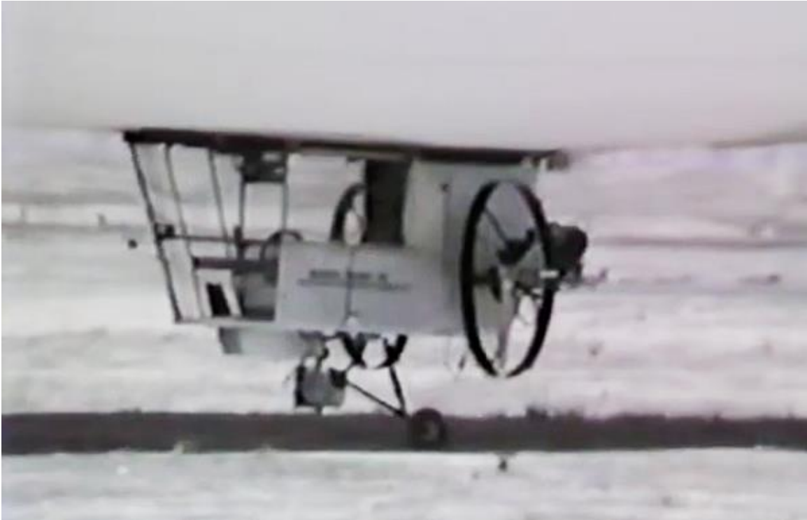
BA-2 gondola with propellers in the cruise (horizontal) position
