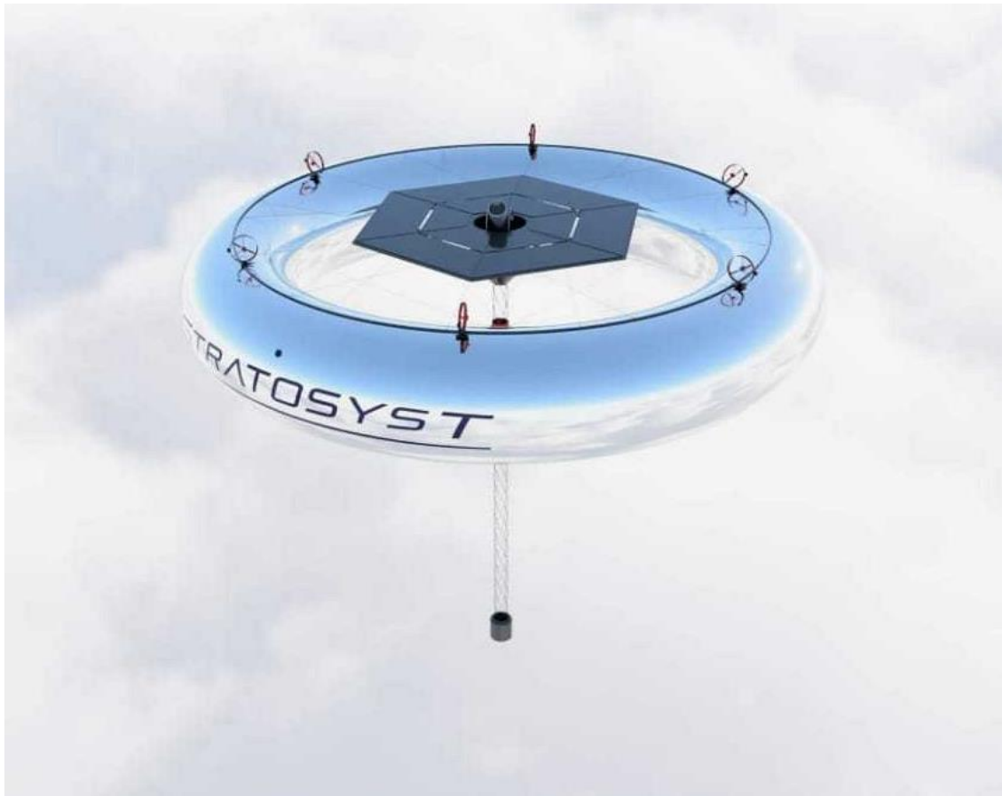
Overhead view of Skyrider in a somewhat different configuration, showing solar panels. Source: Stratosyst (2020)
