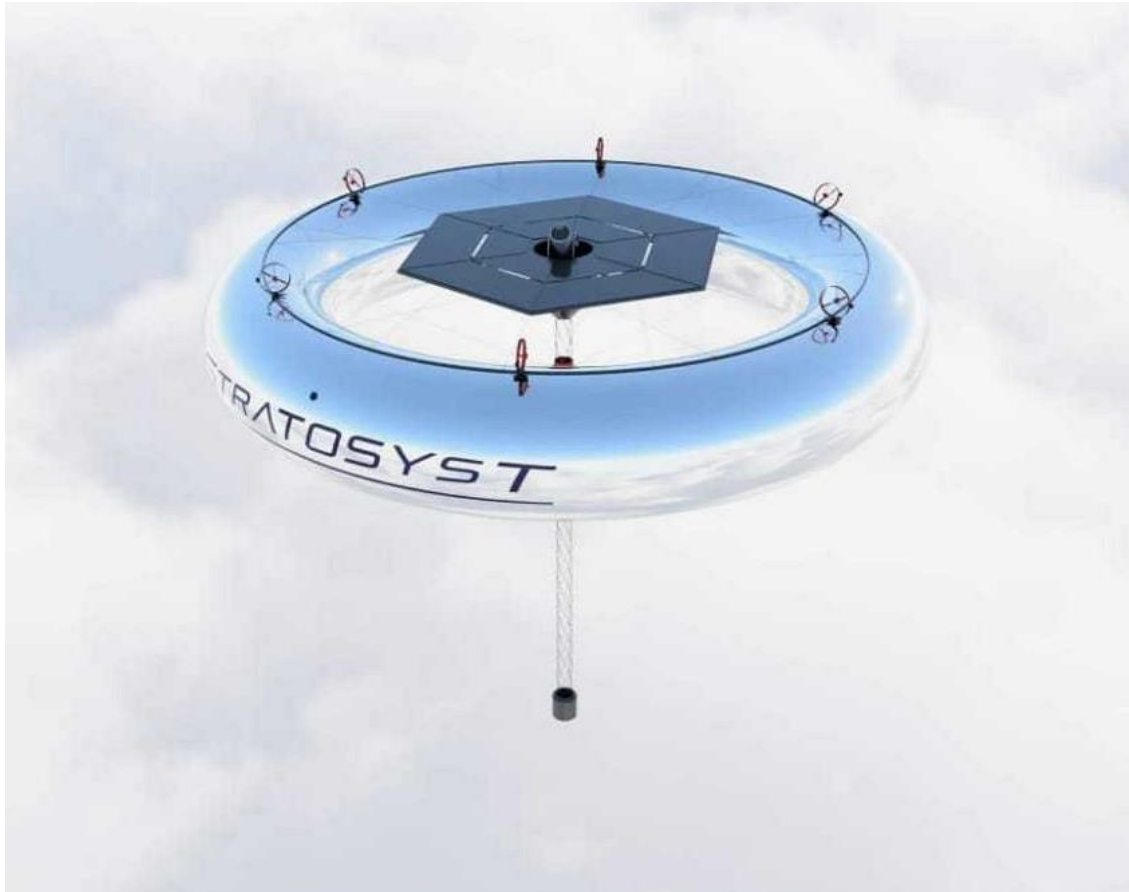
Overhead view of an early Skyrider HAPS configuration, showing solar panels & top-mounted propellers. Source: Stratosyst (circa 2020)
