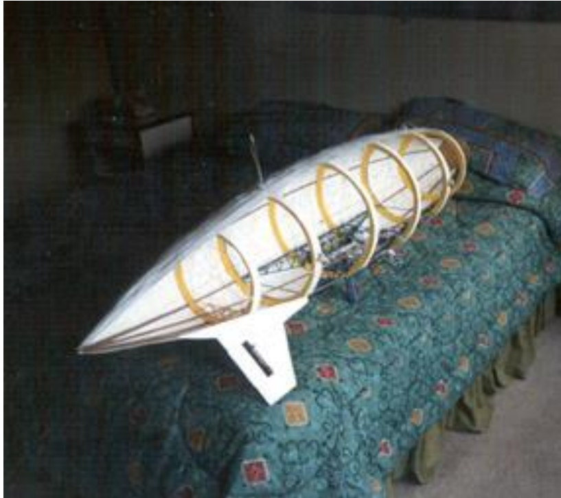
1/100 scale model, view along the starboard side, showing the six internal fabric suspension rings and the placement of two rigid “side girders” and cross beams (black structures).
