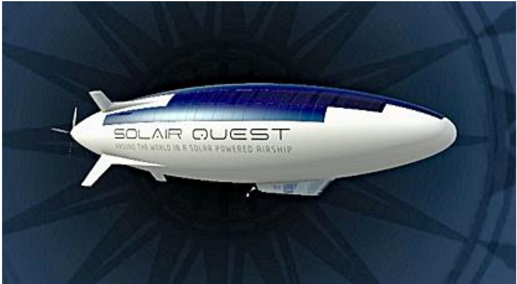
Rendering of Solair Quest semi-rigid, all electric, solar-powered airship. Source: Jesse Blenn
