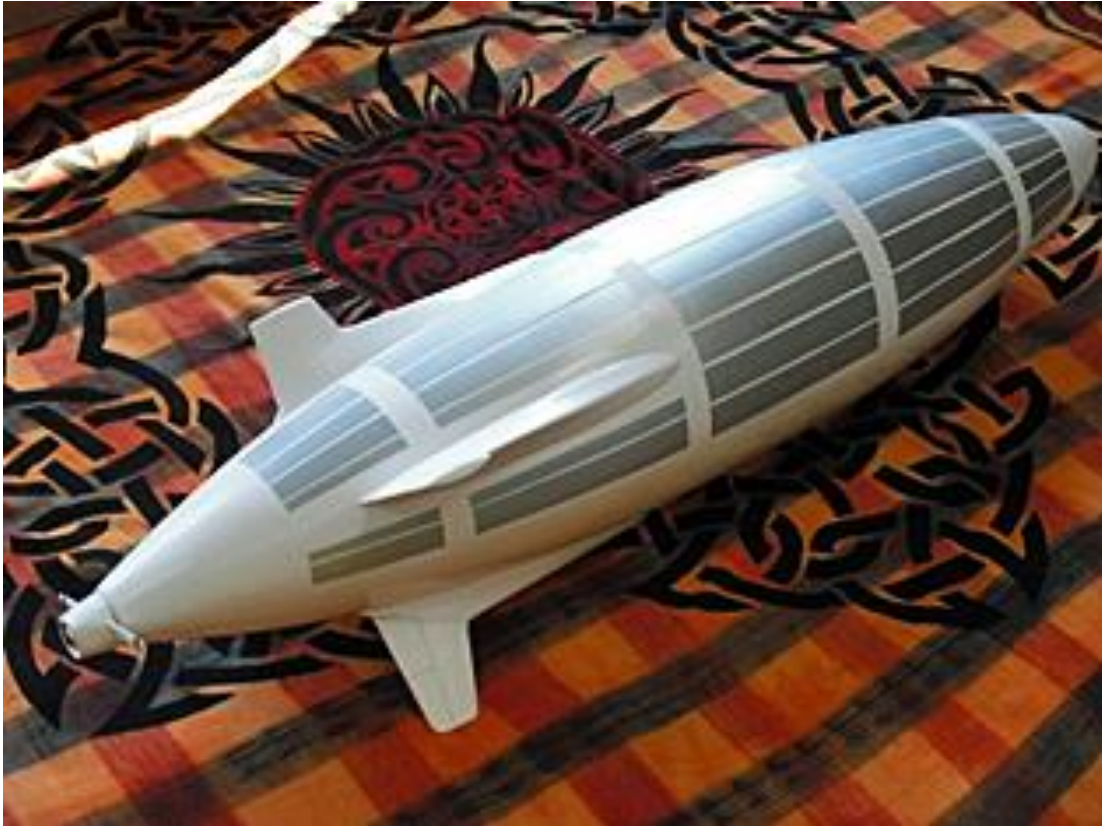
Top view of a scale model of Solair Quest showing the extent of the solar array, X-tail configuration and single tail-mounted propeller. Source: Jesse Blenn
