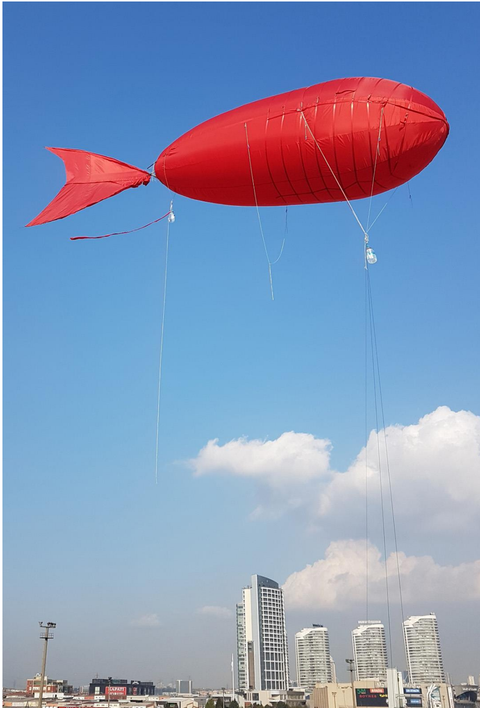
Tethered aerostat. Source: Mustafa Demir
