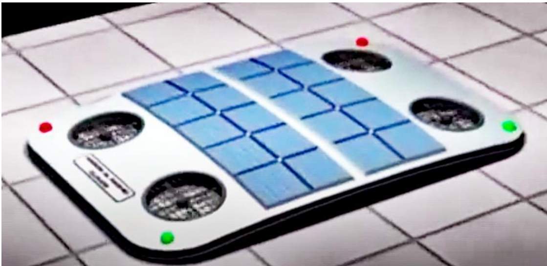
General layout of a Robotic Cloud, showing the four fan propulsors at the corners of the hull and the solar photovoltaic array.
