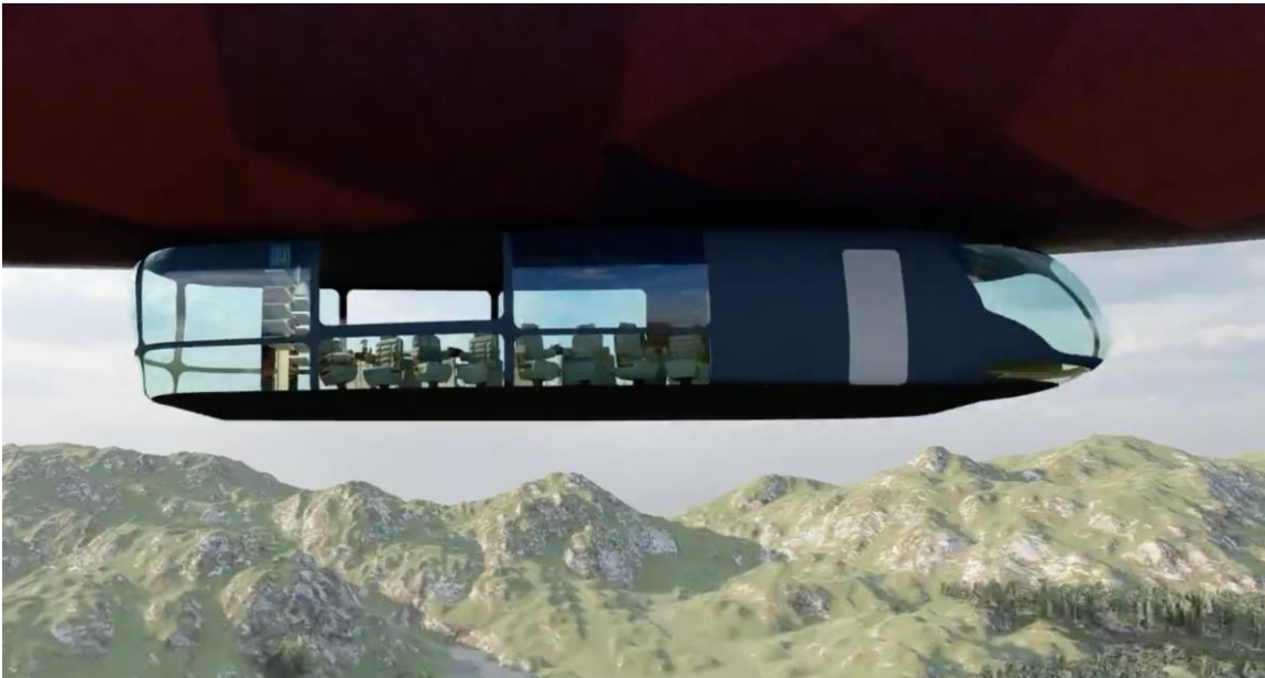
The side view of the gondola shows the three sections: crew cockpit (right), passenger compartment (left), and mid-section service area with boarding door (in white).
