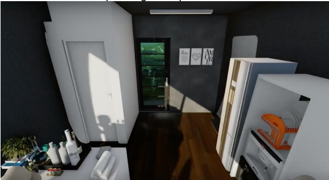
Mid-section service area looking toward the cockpit, showing main boarding door (right), toilet (left) and food and beverage service units. Source, both graphics: Aere (early 2022)
