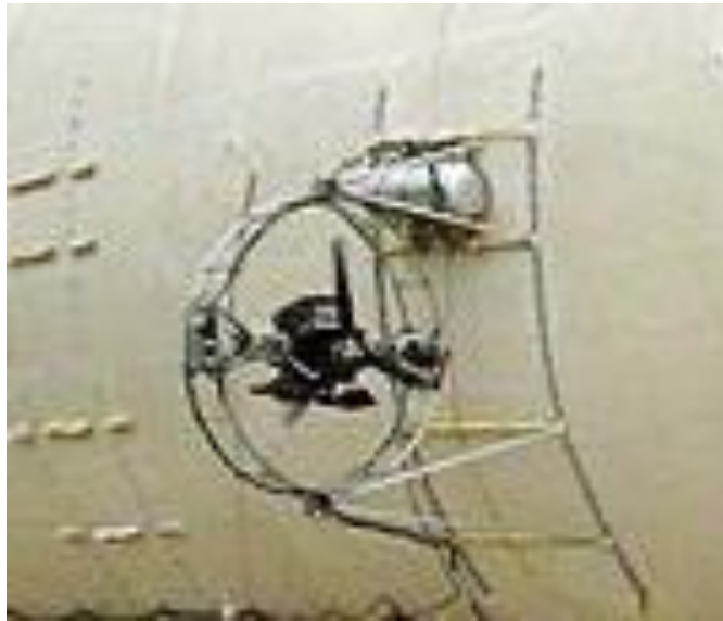
One of two flank-mounted, thrust vectoring, main propellers. Note the support framework attached directly to the envelope. Source, both photos: Chinese Academy of Sciences
