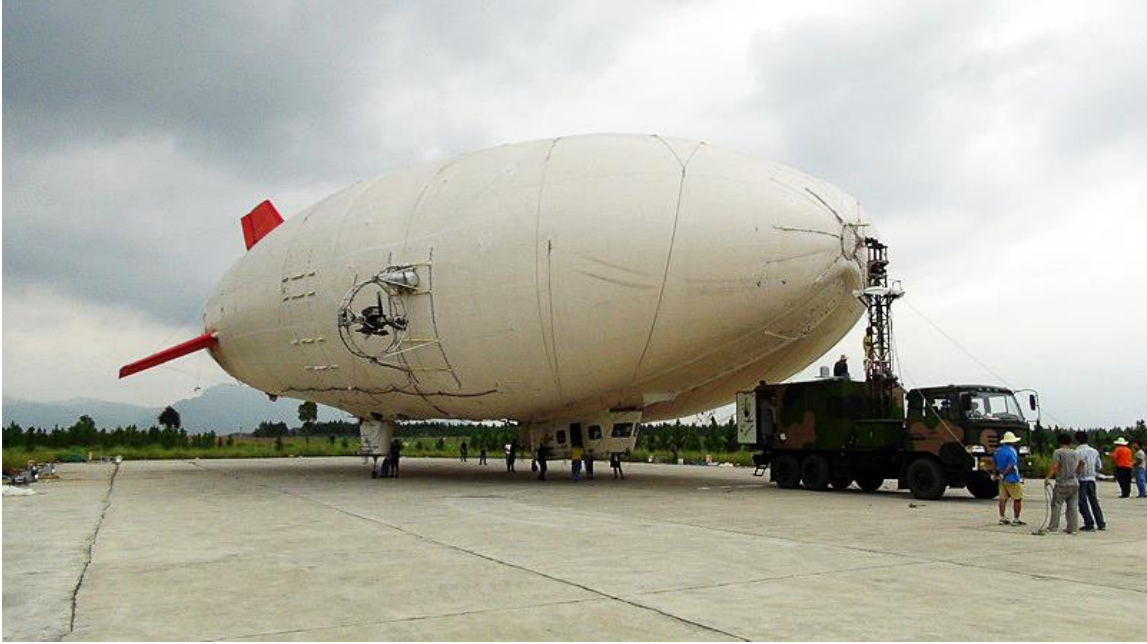
The AEM survey airship on its truck-mounted mobile mooring mast. Note the three-point landing gear, with a nose gear under the central gondola and separate pods under the gas envelope for the main landing gear.
