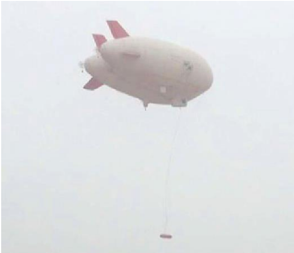
AEM airship in flight with the “bird “ deployed. Source: L. Liu, et al. (2017)
