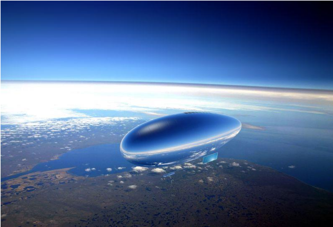
Rendering of the Strasa.Tech HAPS platform at an operating altitude of 18 to 21 km (60,000 to 70,000 ft). Source: Strasa.Tech
