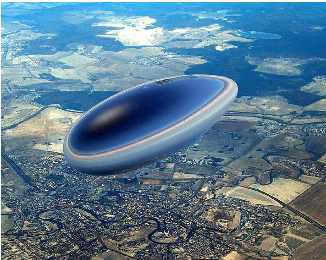
Conceptual HAPS platform configuration has a tailless, non-rigid, superpressure gas envelope carrying a small suspended gondola with two electric-powered propellers, and two solar arrays (top of envelope & suspended panel). Source, both graphics: Strasa.Tech
