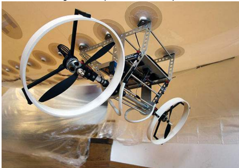
Minimal “gondola” on the Aero Drum aerial photography blimp. The array of reinforced mounting pads on the Aero Drum blimp allows the gondola and payload package to be positioned longitudinally to manage the center of gravity of the blimp. Source: Aero Drum Ltd. & Challenger Aerospace via aeroexpo.online
