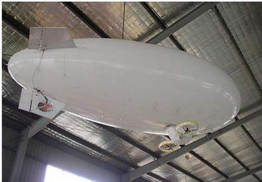
A Challenger Aerospace UAS standard blimp showing placement of a modular gondola with main propulsors positioned for vertical thrust, a single main landing wheel, and the cruciform tail with aerodynamic control surfaces and lateral thruster. Source, both photos: Challenger Aerospace
