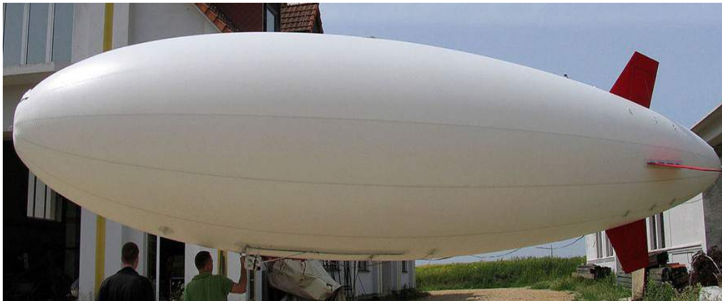
10-meter Aero Drum aerial photography blimp. Source: Challenger Aerospace
