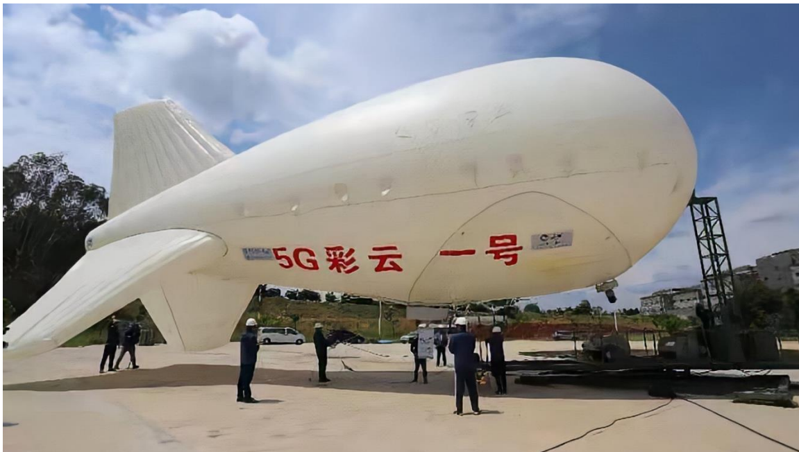
The 5G Cloud One aerostat on its mooring mast, with a 5G antenna under the envelope.
