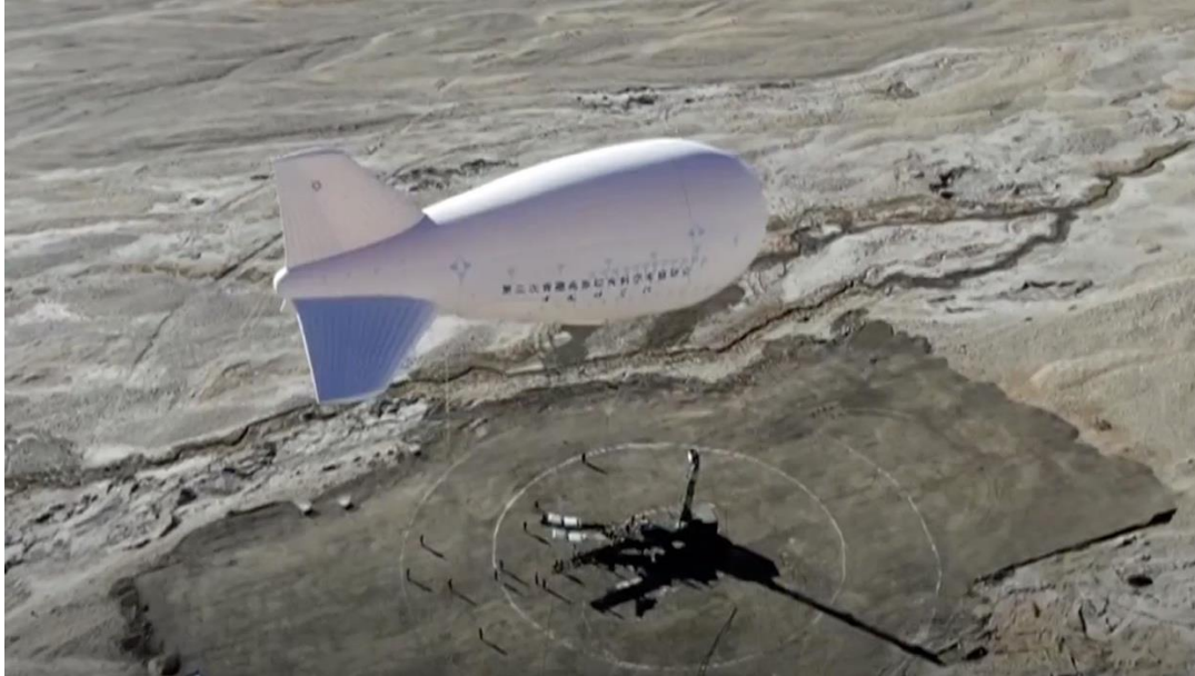
Jimu No.1 tethered and flying above the mooring platform.
