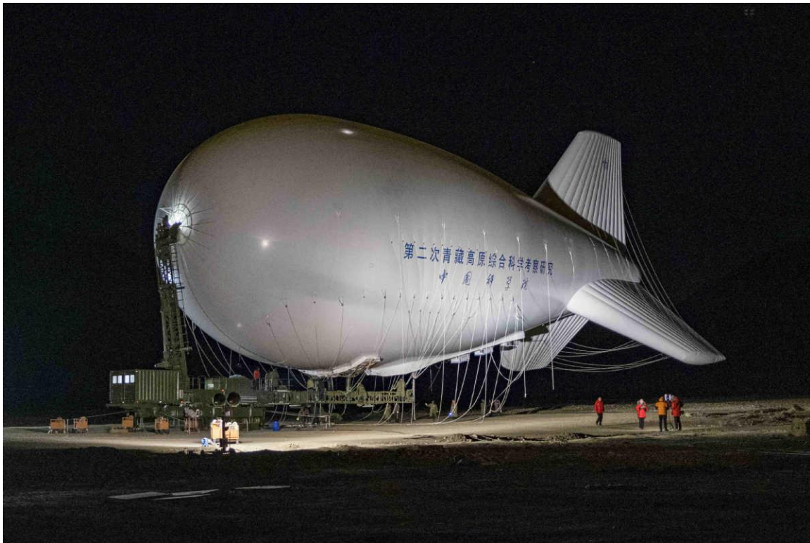
Jimu No.1 at its mooring tower prior to a night launch. Source: SUN Fei/Xinhua
