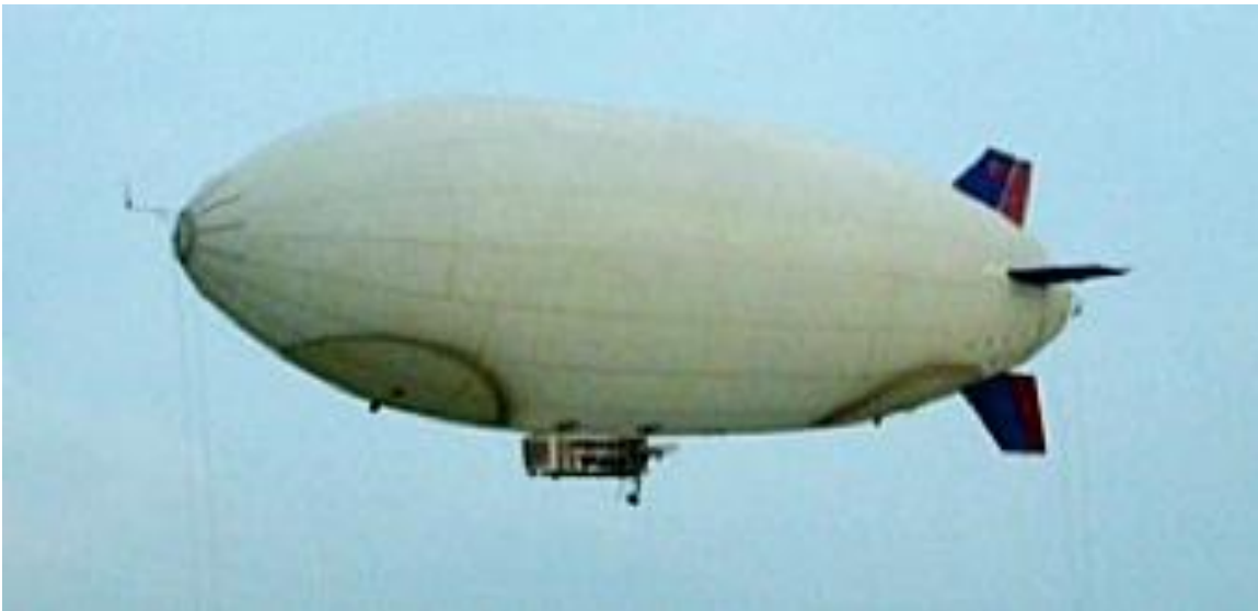
Zhiyuan-1 airship flight, showing the darker outlines of the ballonets inside the envelope. Note that the shrouded propellers on the gondola are vectored horizontally to provide lift.
