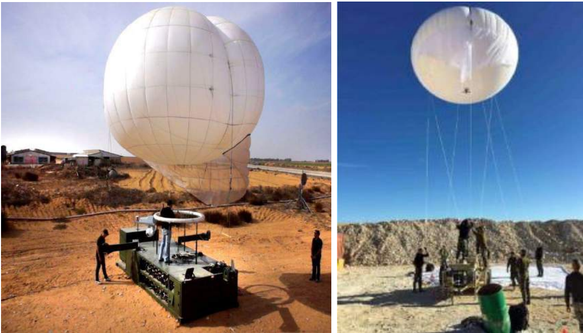
SAS tethered balloon field launch. Source, both photos: SAS
