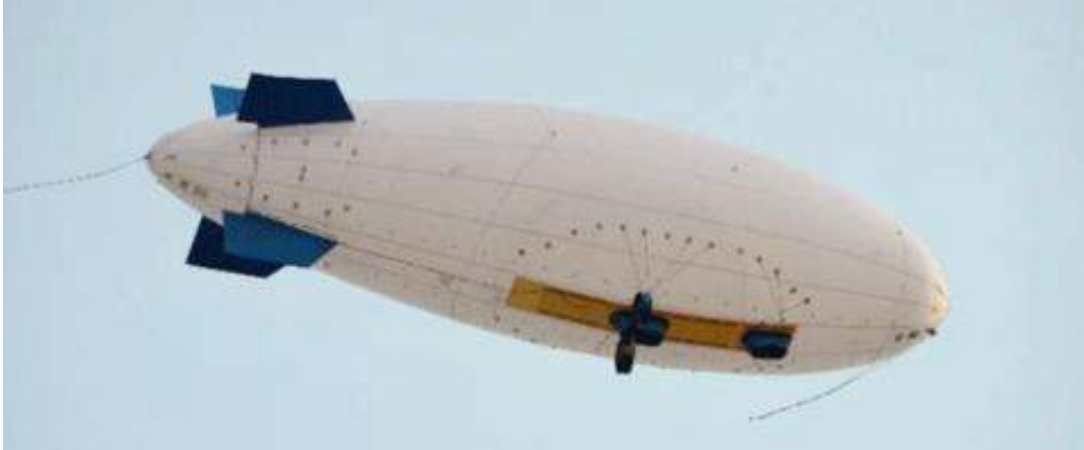
FZ-series ZH-A300. Note the elliptical array of reinforcement points around the bottom of the envelope for attaching the supporting cables for the gondola and separate payload modules. Also note the elliptical array of reinforcements for the tail fin support cables.
