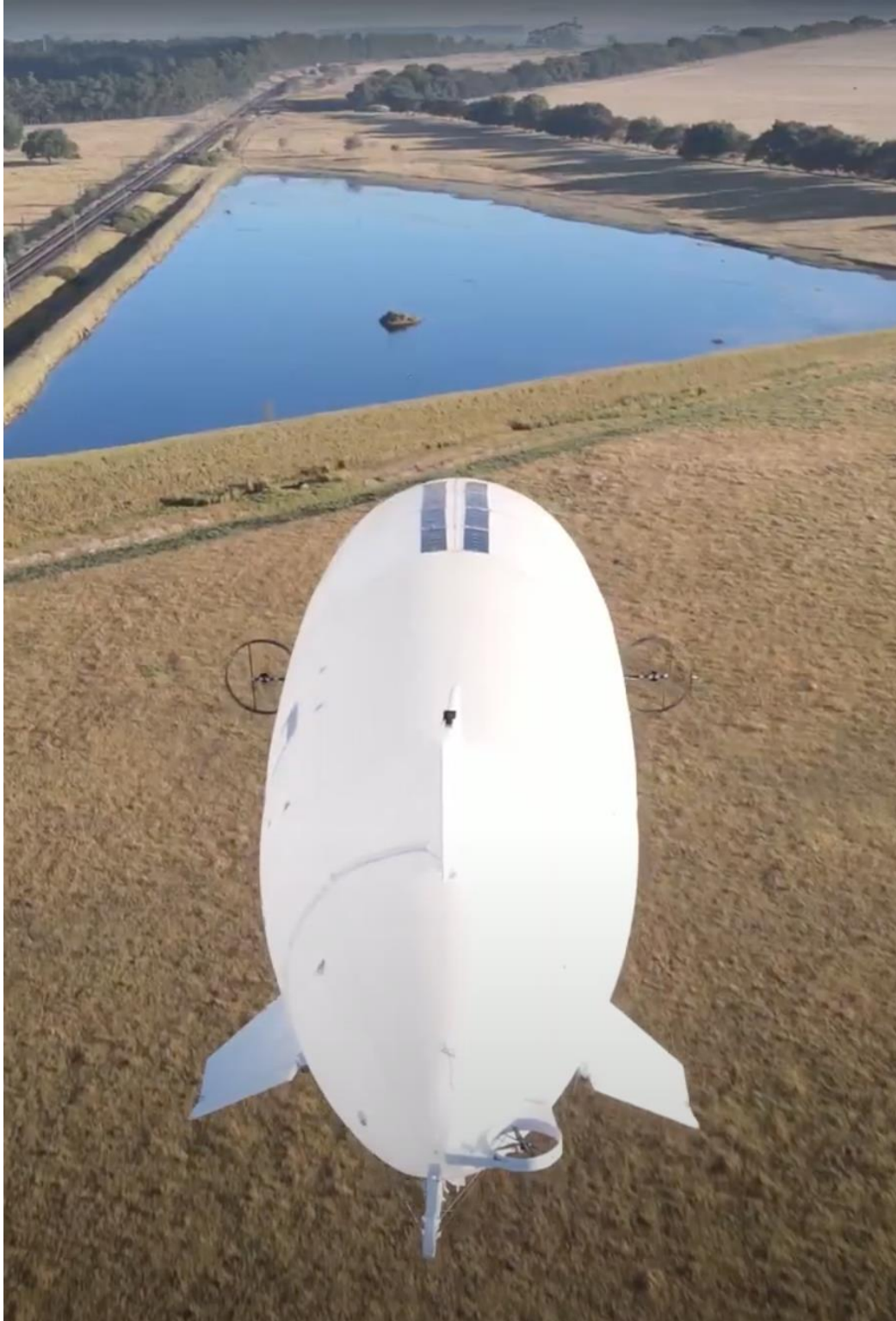
Stern overhead view of the production prototype, showing the placement of the shrouded main propellers and the stern maneuvering thrusters. Note the control surfaces on the inverted Y-tail fins. Source: Screenshot from Cloudfline video (2022)
