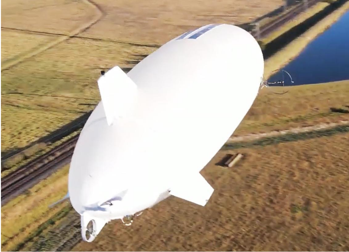
Note the shrouded main propeller vectored for cruise thrust.
