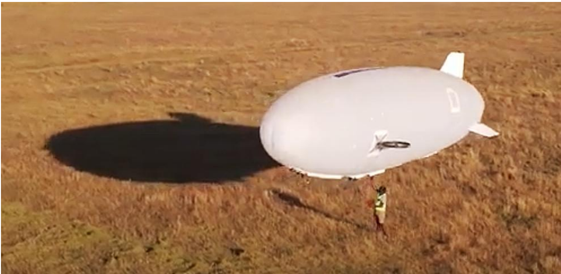
The Cloudline production prototype hovering. Note the shrouded main propeller vectored for lift. Source: Screenshot from Cloudline video (2022)
