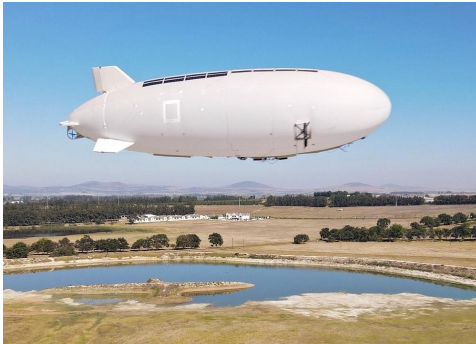
Side view of the production prototype showing a shrouded main propeller vectored for cruise propulsion. The inverted-Y tail has movable aerodynamic control surfaces, which provide maneuvering control during cruise flight. Source: Screenshot from Cloudline video (2022)
