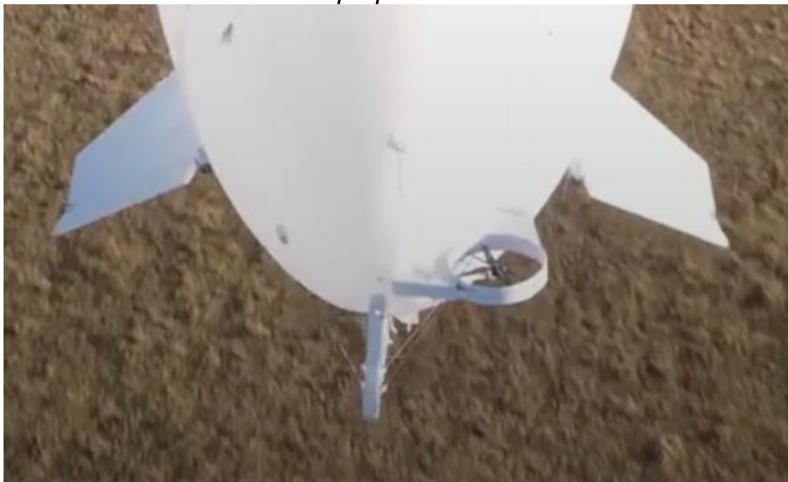
Stern views of the production prototype showing the lateral and vertical thrusters used for low speed maneuvering, when the aerodynamic control surfaces lose their effectiveness.
