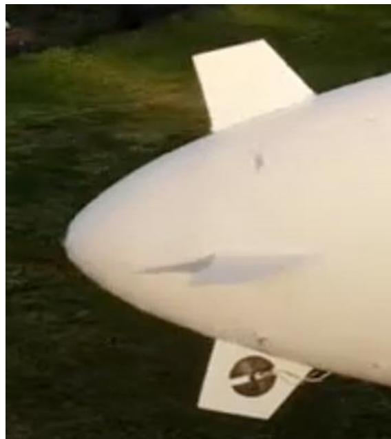
(R) Stern view showing the cruciform tail fin configuration and the lateral thruster in the lower fin for high maneuverability at low speed.
