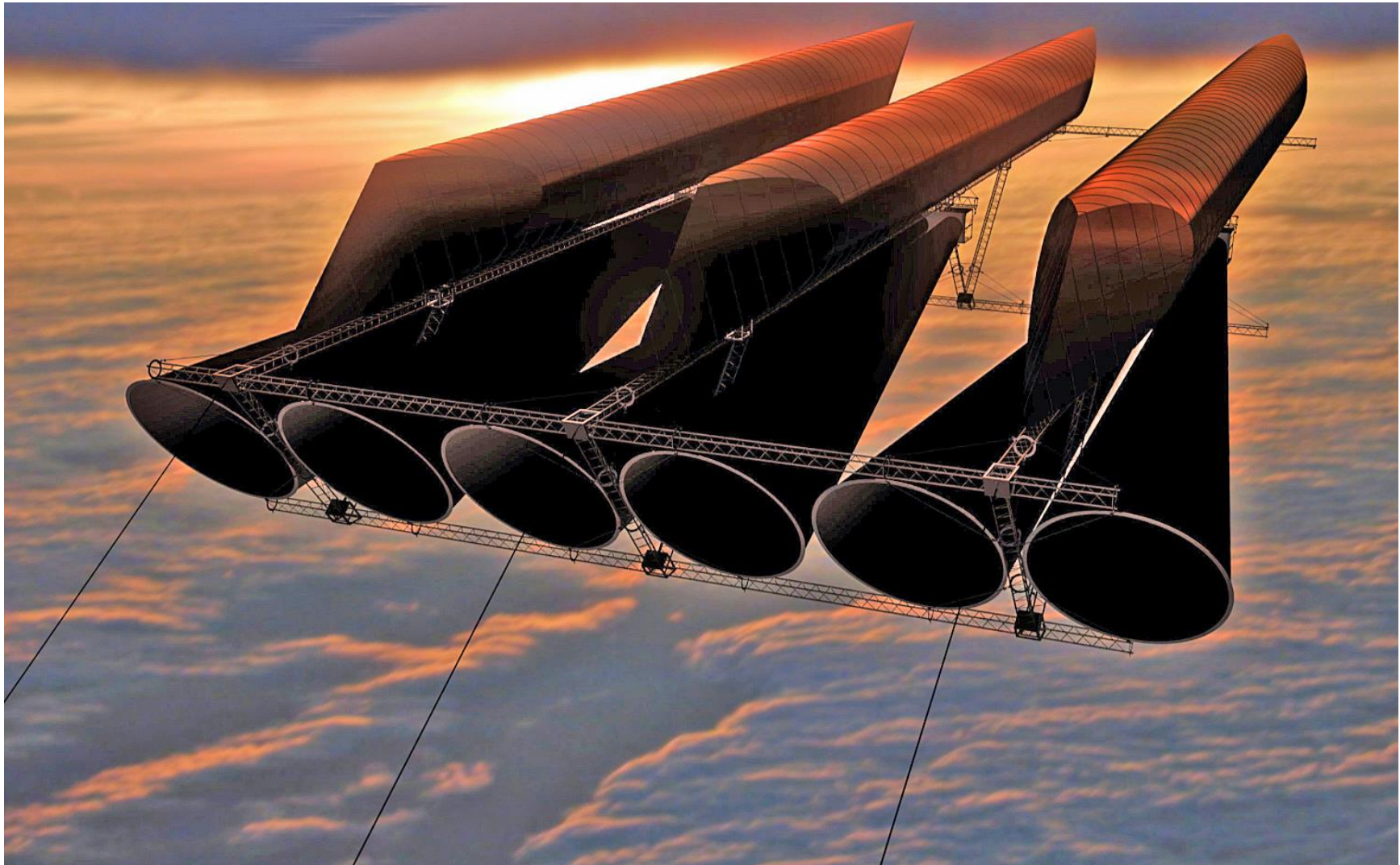
Rendering showing the general arrangement of an Airbine™ module comprised of three platforms, each with two air funnels. Note the rigid transverse truss framework connecting the three platforms at their front and back, and the three tethers connected to the front truss framework. Source: ARES
