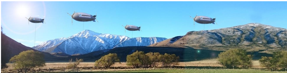
Four tethered aerostat wind generators deployed in a rural setting.
