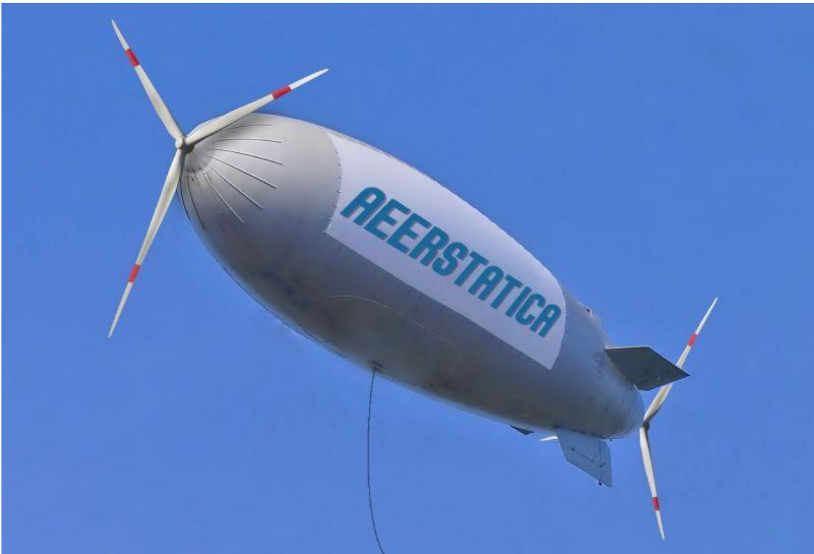
Aerstatica's tethered aerostat wind generators face into the wind when deployed, with the bow and stern rotors rotating in opposite directions. Source, both graphics: Aerstatica Energy Airships
