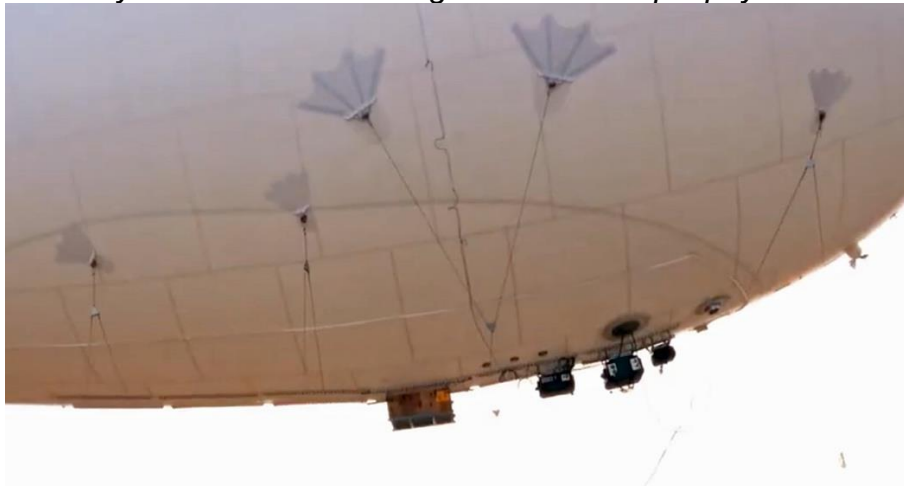
Multiple payloads installed under the aerostat gas envelope.
