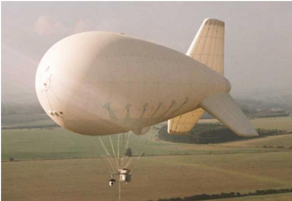
An Airborne Industries 19-meter (400 m 3 ) operational aerostat in flight with a suspended payload. Source: Airborne Industries
