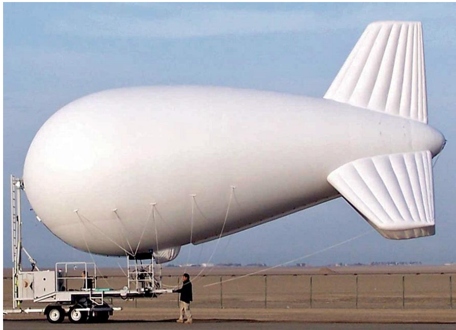
An Airborne Industries 15-meter (210 m 3 ) tactical aerostat on its mobile ground handling system. Source: Airborne Industries
