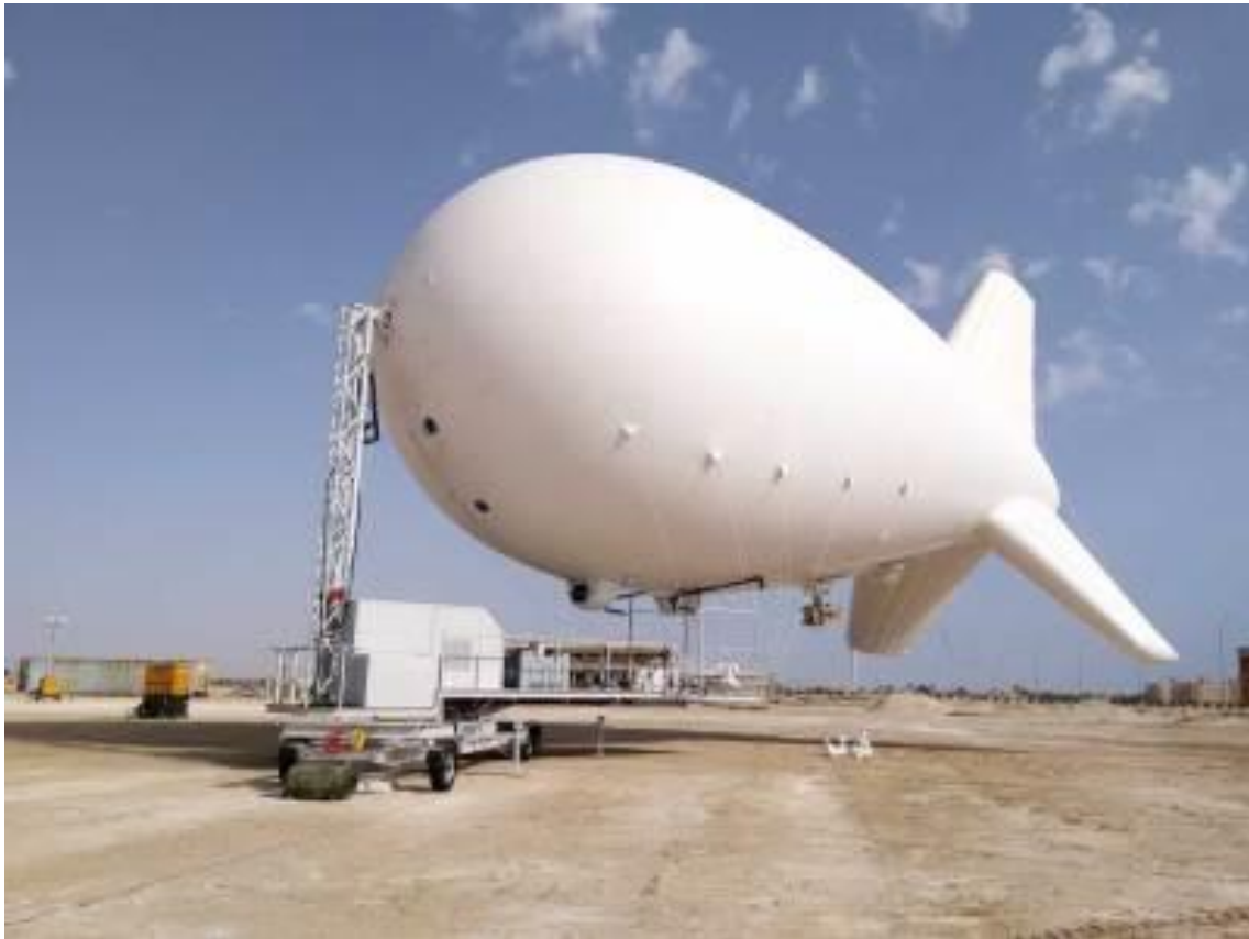
An Airborne Industries 850 strategic aerostat on its mobile Ground Handling System. Multiple payload modules are attached along the bottom centerline of the gas envelope. Source: Airborne Industries
