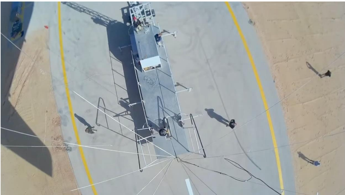
View of the mobile Ground Handling System from an 850 Persistent Ground Surveillance System. Source: Screenshot from Airborne Industries video.
