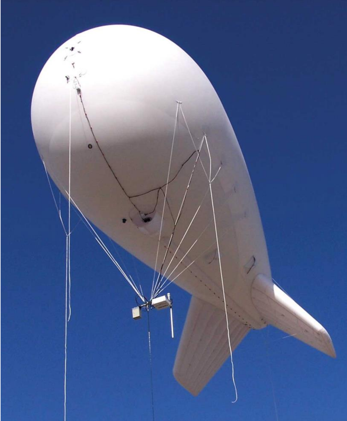
An Airborne Industries 15-meter (210 m 3 ) tactical aerostat in flight. Source: Airborne Industries
