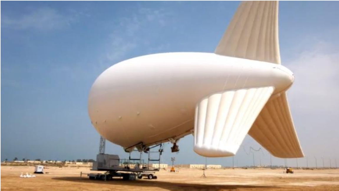
An Airborne Industries 850 strategic aerostat on its Ground Handling System. Source: Airborne Industries
