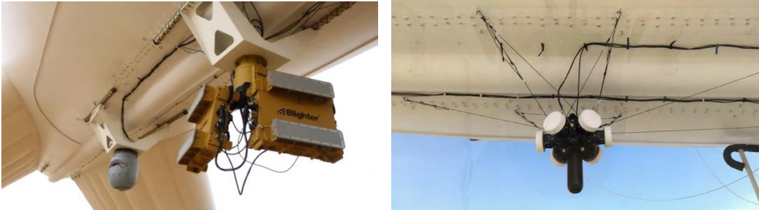
(Left) EO/IR turret and rotating radar antennas. (Right) Listening device antenna. Source: Screenshots from Airborne Industries video
