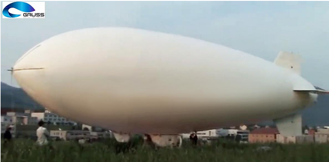
Bow quarter view of a Gauss 20-m blimp with cruciform tail.
