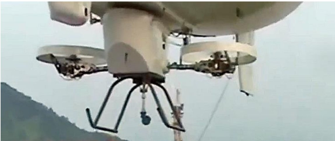
Gauss 20-m blimp gondola housing the propulsion system with two cantilevered, shrouded, thrust-vectoring propellers (shown vectored up for lift during takeoff). A mission module is attached forward of the gondola. Both are attached via a reinforced rail system along the bottom of the envelope. Source: Screenshots from Gauss 20-m blimp video (2022)
