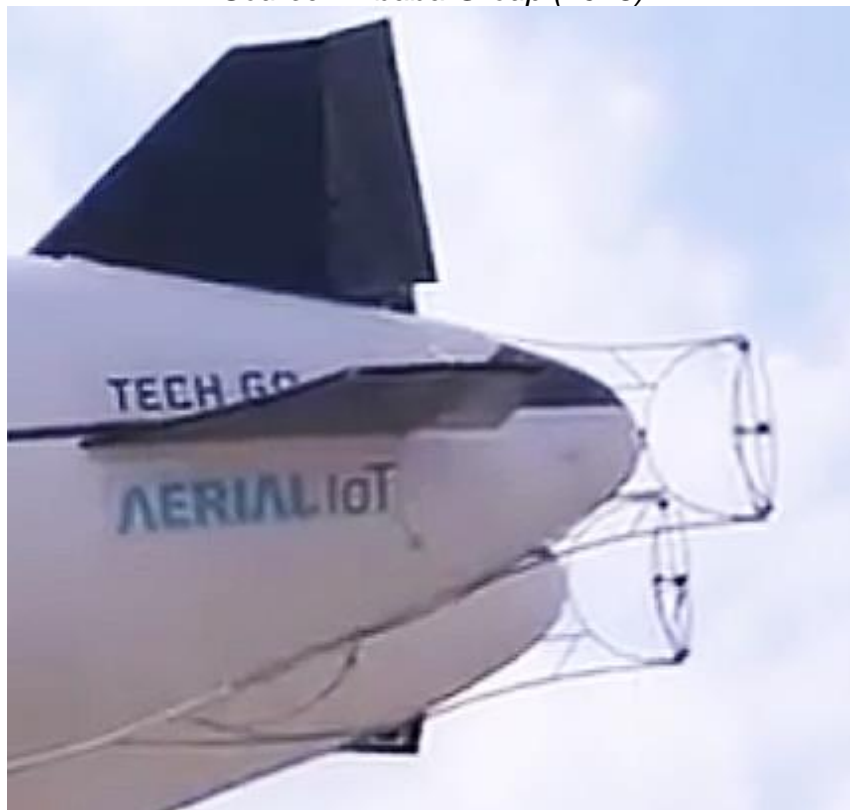
Stern thrust-vectoring propellers. Source: The Morning Context (May 2022)
