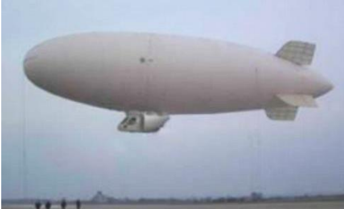
Gauss 30-m unmanned blimp with internal propeller. Source: Gauss
