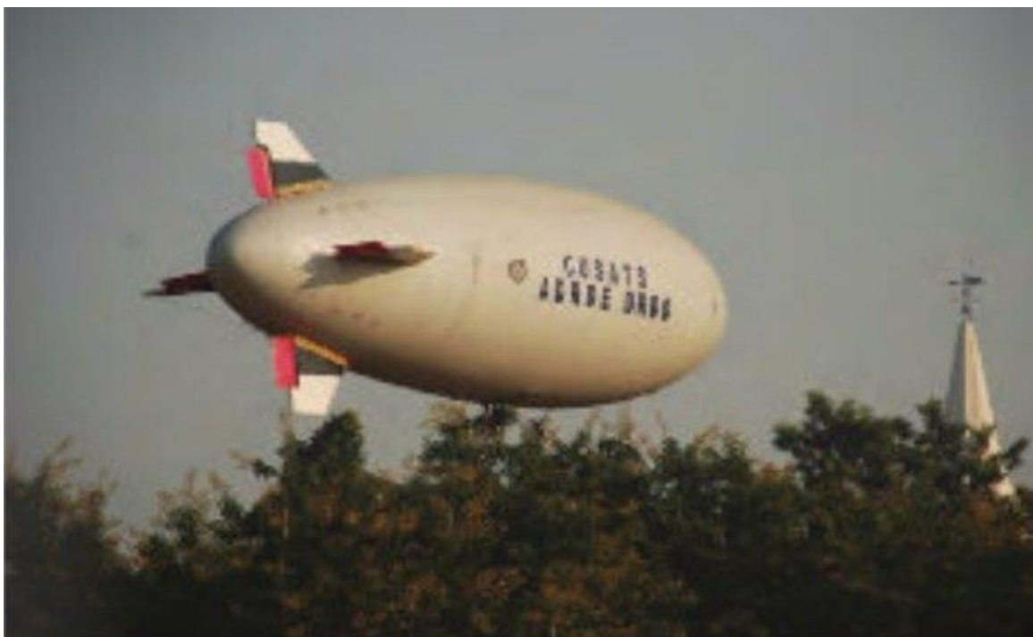
USAS sub-scale prototype. Note the red rudder and elevator control surfaces on the cruciform tail fins. Source: Defense India Twitter (24 Jun 2018)
