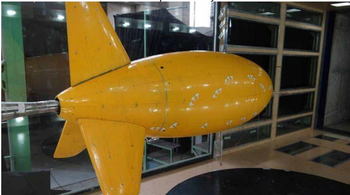
Model of DRDO's Akashdeep aerostat during wind tunnel testing. Source: DRDO via Strategic Frontier
