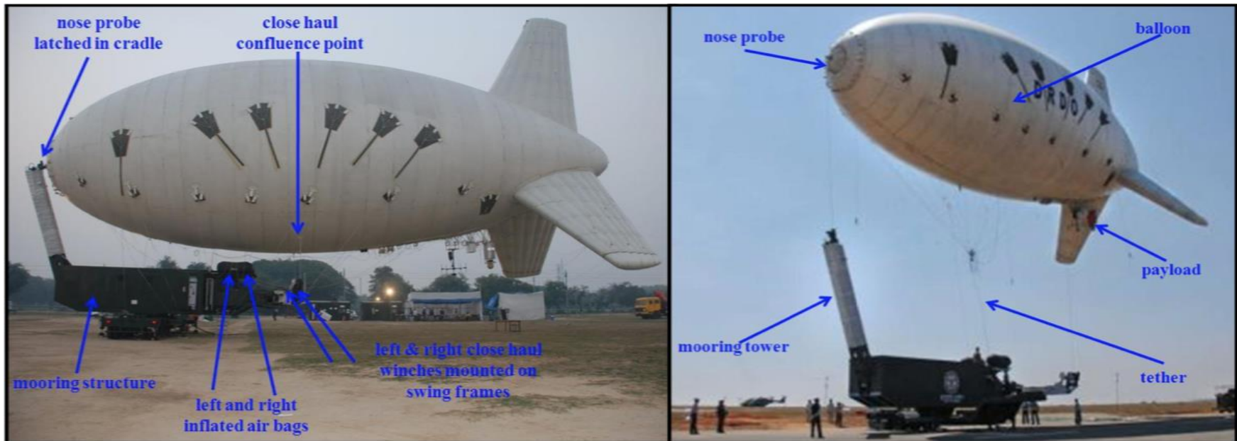
Akashdeep tethered aerostat, moored (left) and being deployed (right). Source: A. Kumar, et al., IJMET (2013)
