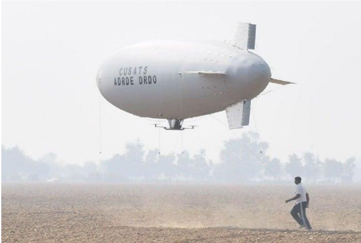
USAS sub-scale prototype. Note the two thrust-vectoring propellers (vectored up) cantilevered from the small midships gondola. Source: India Defence Forum (Jan 2019)
