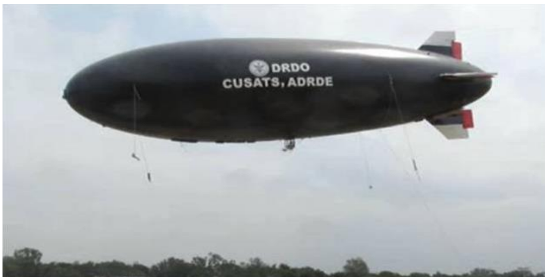
USAS sub-scale prototype with a small gondola amidships. Source: DRDO
