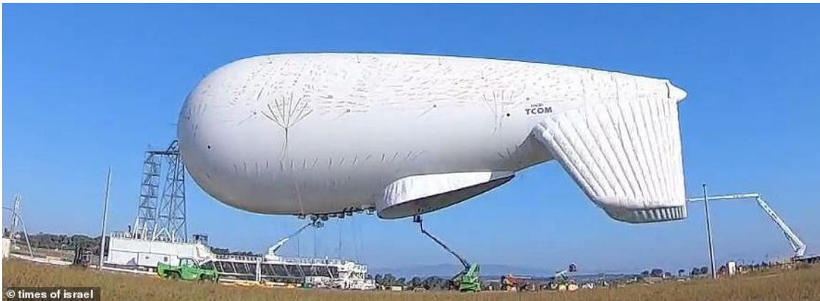
HAAS aerostat at its mooring platform before installation of the windscreen (radome) and inflation of the tail fins.
