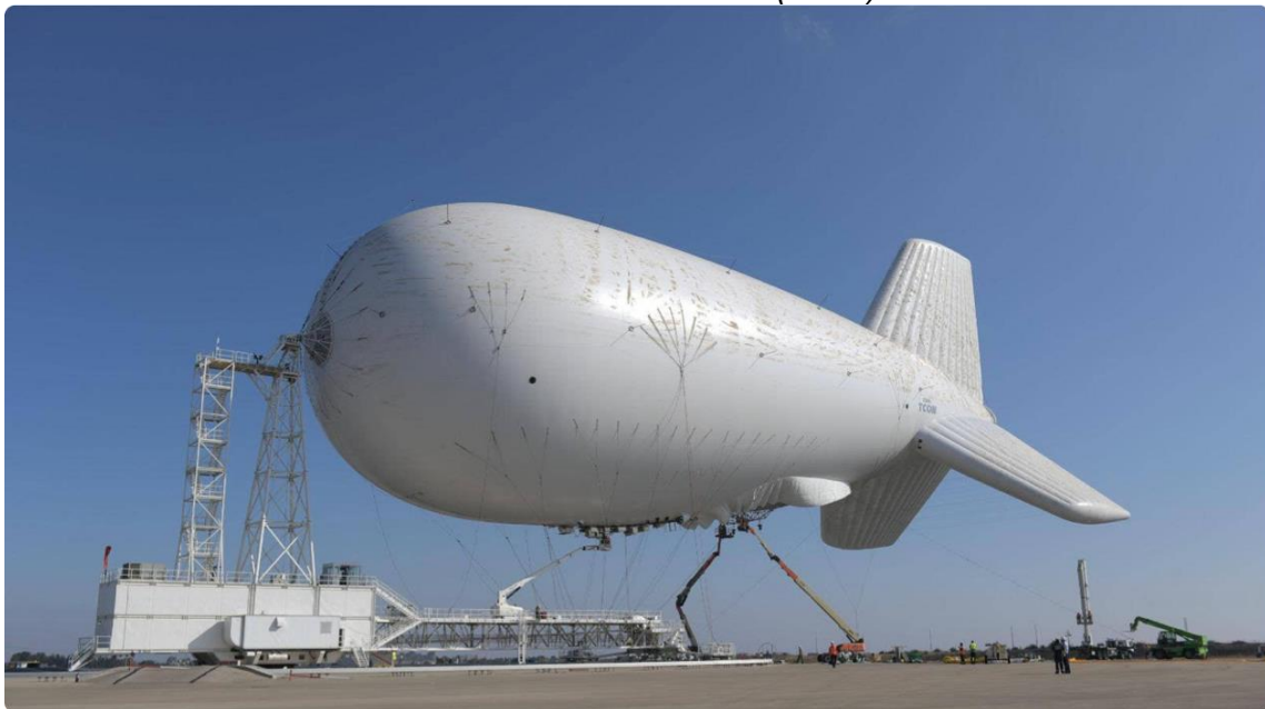
HAAS aerostat at its mooring platform before installation of the Windscreen. Source: Ministry of Defense, Israel
