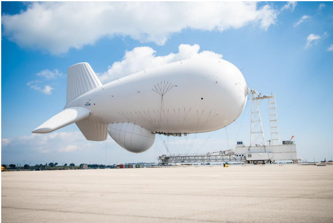
HAAS aerostat at its mooring platform with the airborne radar installed. Source: The Defense Post (2022)
