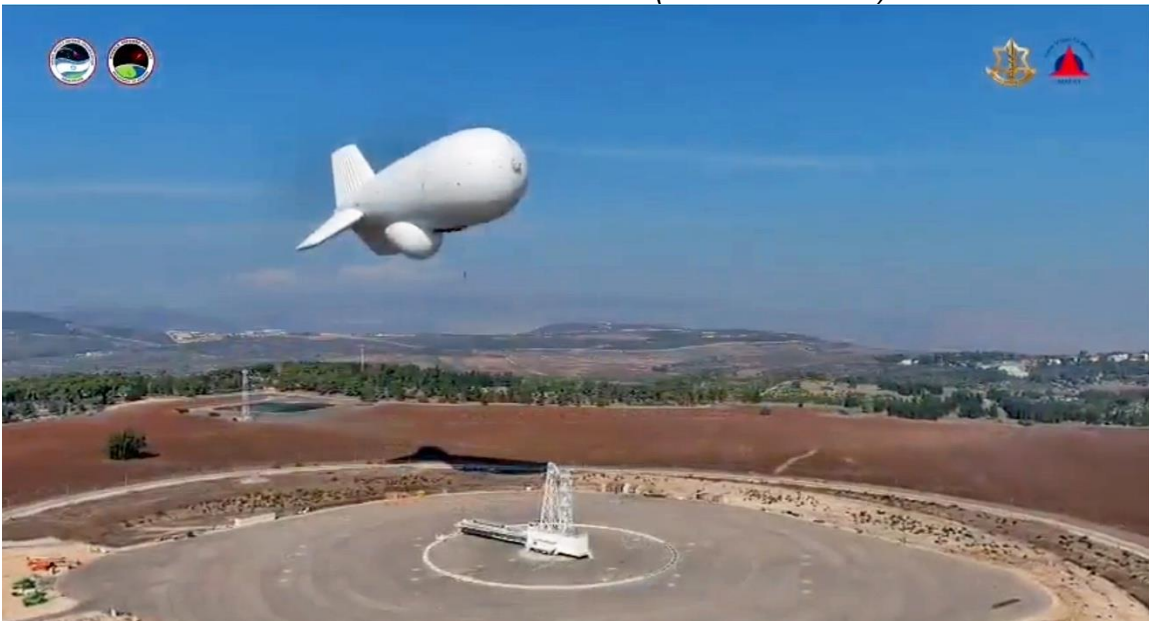
HAAS aerostat aloft, above its mooring platform. Source: Screenshot from TCOM video (2022)
