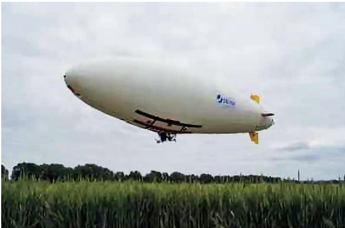
Jülich Fieldship UAV blimp in low-level flight. Source: Jülich Institute
