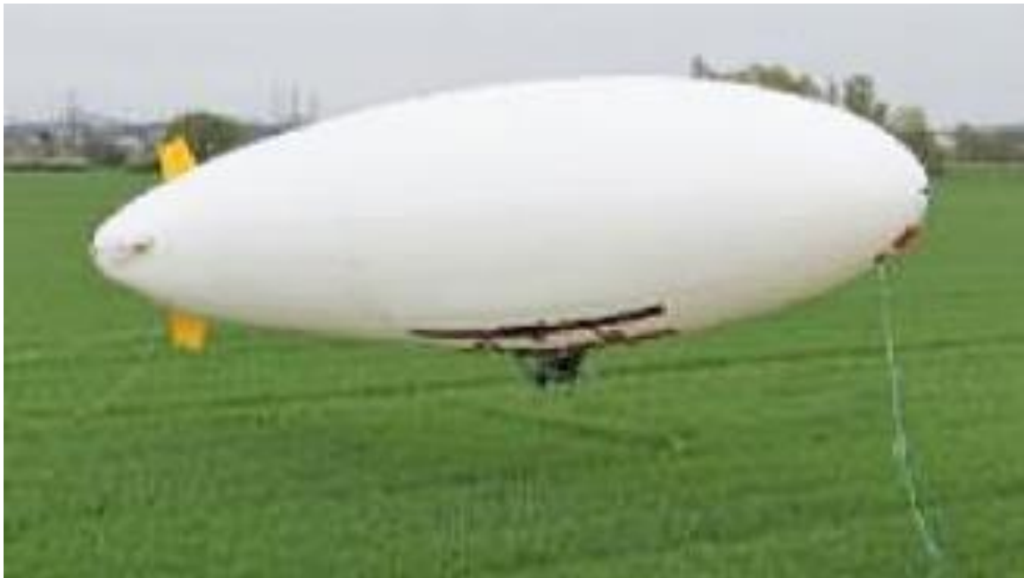
Jülich Fieldship UAV blimp. Source: Jülich Institute
