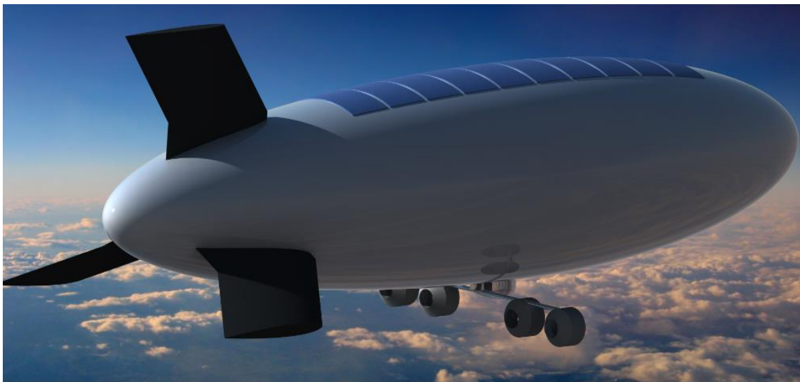
Rendering of a Tepegöz unmanned, autonomous airship, stern quarter view. Source: Otonom Teknoloji
