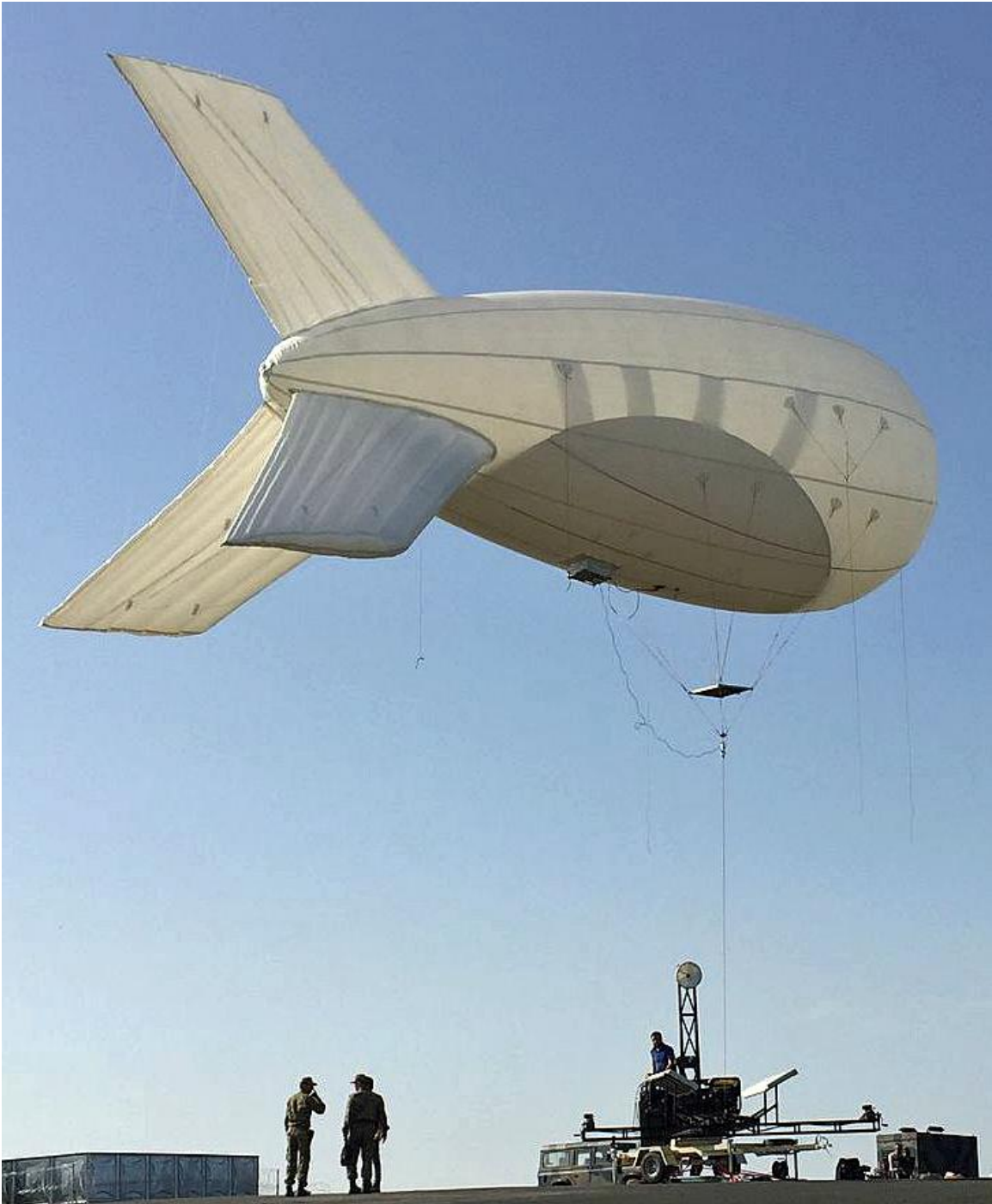
A Doruk 133B tactical aerostat above its mobile mooring station. Note the shadow of the ballonet inside the gas envelope. The small rectangular platform suspended from the envelope supports the payload module. Source: Otonom Teknoloji
