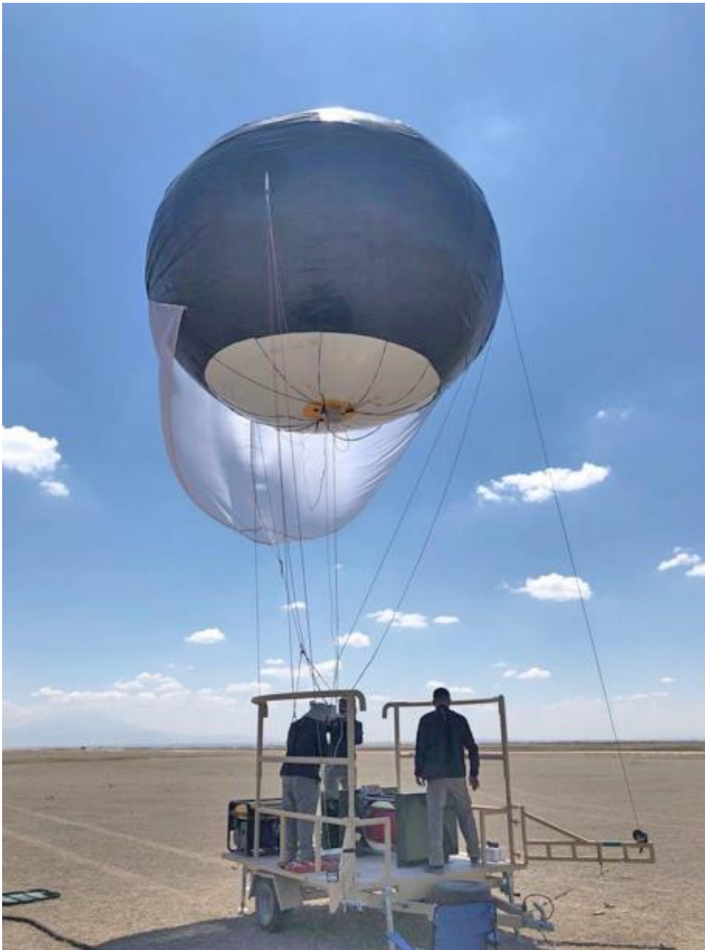
Dolunay aerostat on its mobile launcher. Black gas envelope provides a larger infrared signature for use as a target balloon. Source: Otonom Teknoloji
