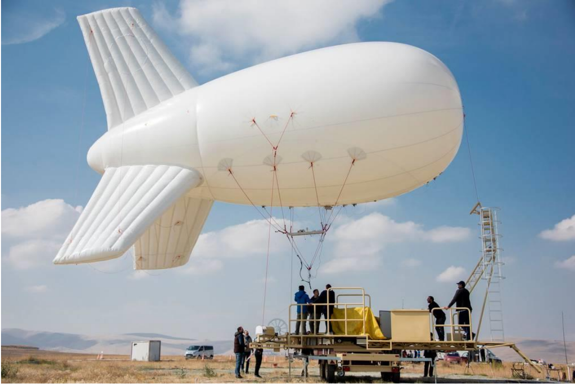
A Doruk operational aerostat on its mobile mooring station. Source: Defence News (2021)
