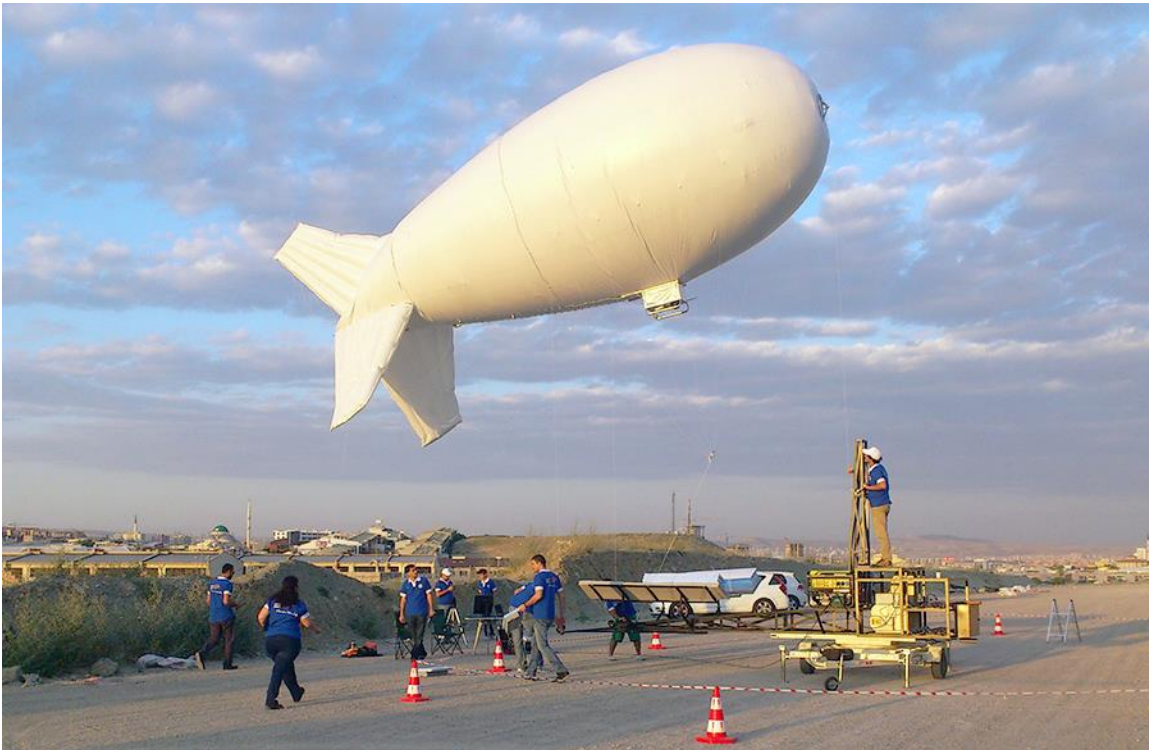
Doruk prototype in flight above its mobile mooring station. Source: Otonom Teknoloji (2014)
