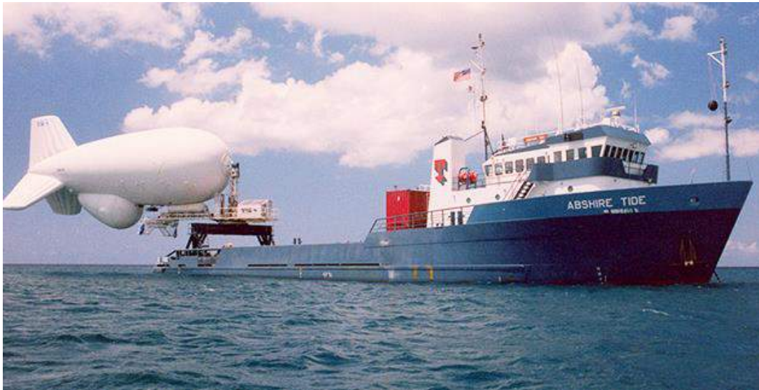
Army SASS ship Abshire Tide with TCOM 25M aerostat. Source: TCOM LP
