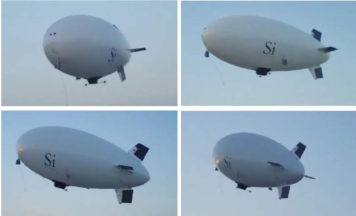
Altus fly-by during flight testing as a free-flying drone blimp. Note the cruciform tail fins with active flight control surfaces. Source: Screenshots from Silicis video (17 November 2010)
