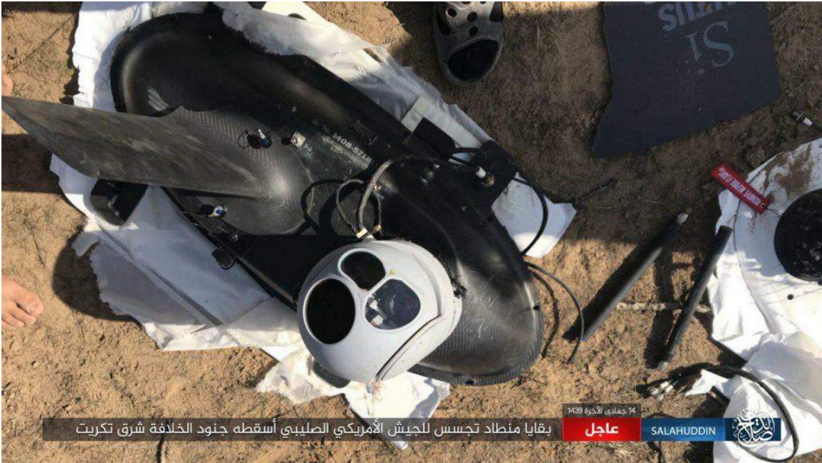
One Altus was reported to have been shot down by ISIS fighters in March 2018. This is the EO/IR camera and antenna module for the recovered Altus. Source: Defence Blog (3 Mar 2018)
