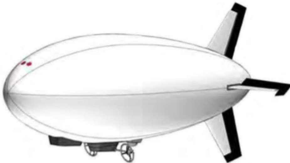
General arrangement of an Altus free-flying drone blimp. Source: DoD Summary Report (2012)
