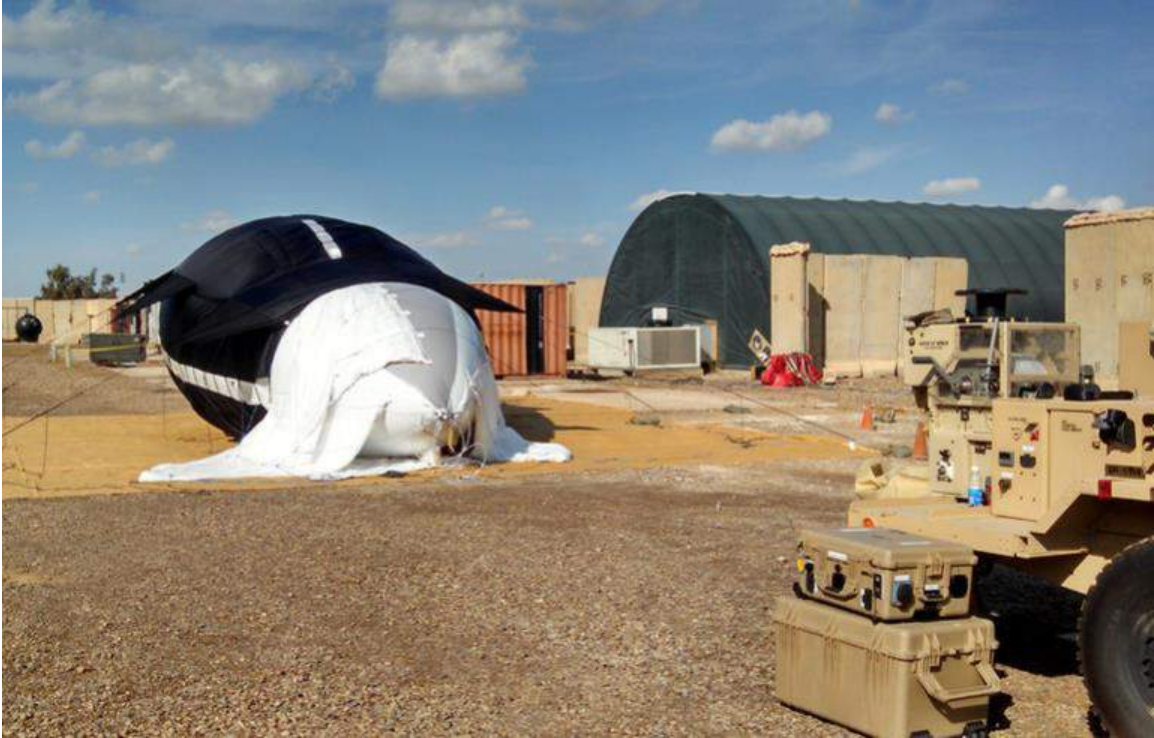
Altus aerostat secured on the ground between missions. Source: Silicis
