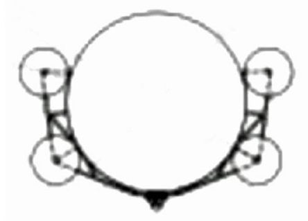
Front view, showing cantilevered transverse propulsion pylons supported from the rigid keel and fitting closely around the gas envelope
