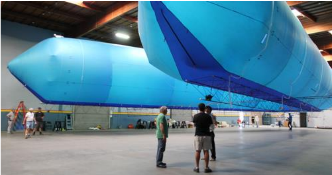
Ascender 28 float test. Note the visible carbon fiber keels outside the V-shaped gas envelope. Source: JP Aerospace
