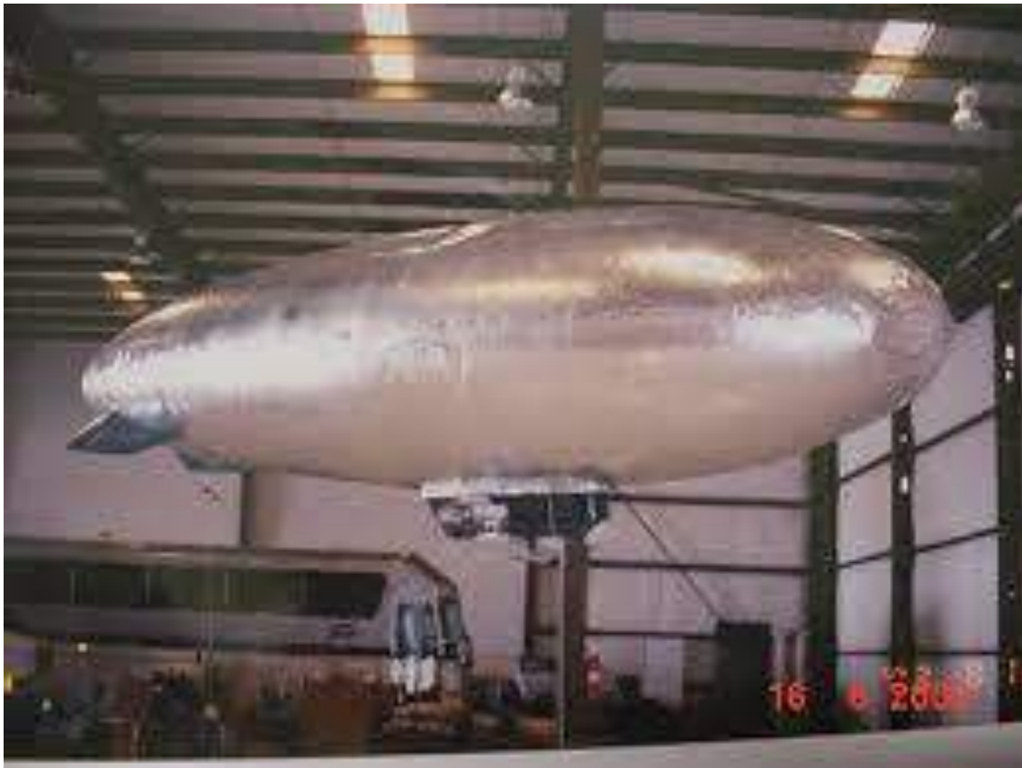
23-foot (7-m) long, remote controlled, helium blimp manufactured by Airspeed Airships and adapted for cycloidal propeller testing by Roy P. Gibbens. Note that the upper tail fins have been removed. Source: Gibbens (photo 2001)
