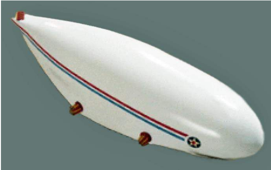
AirLighter 2 model bow overhead view showing two flank-mounted cycloidal propellers and one more aft, atop the tail for precise low-speed directional control. Source: Roy P. Gibbens (2003)
