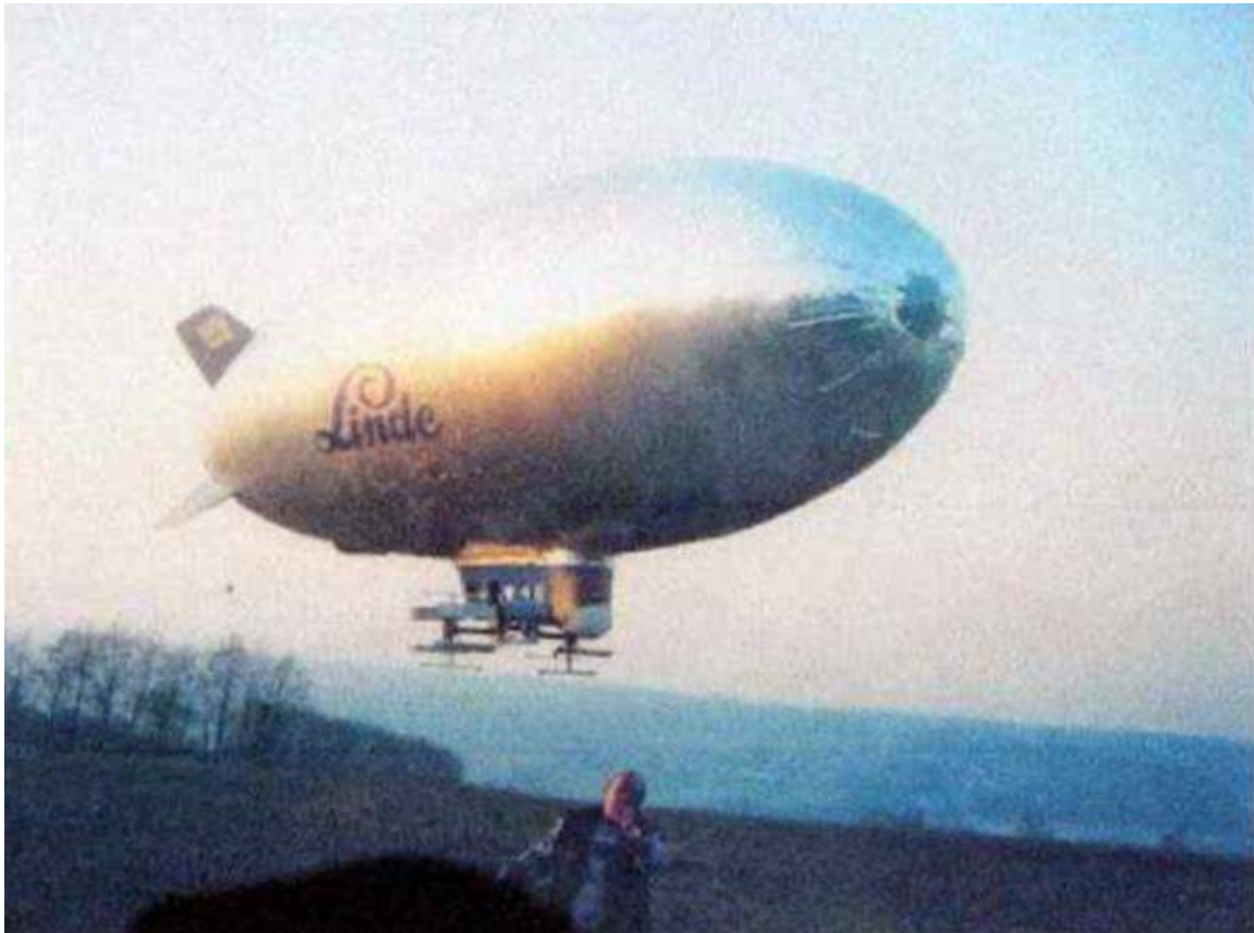
A 7 m (23 ft) Airspeed Airships blimp, likely an AS-300, adapted for testing cycloidal propellers. Source: Roy Gibbens (2011)
