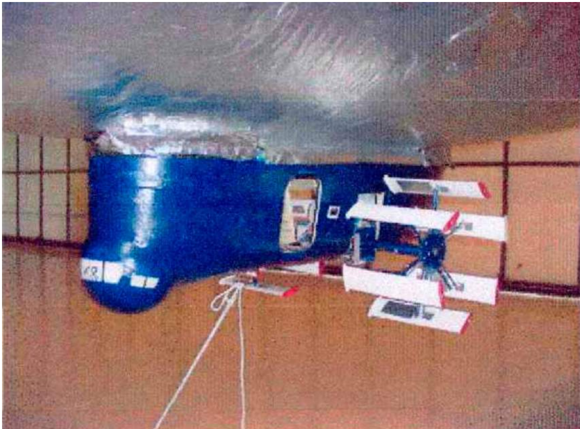
Cycloidal propeller installation on a remotely-controlled blimp. Source: Roy P. Gibbens DARPA white paper, circa 2008
