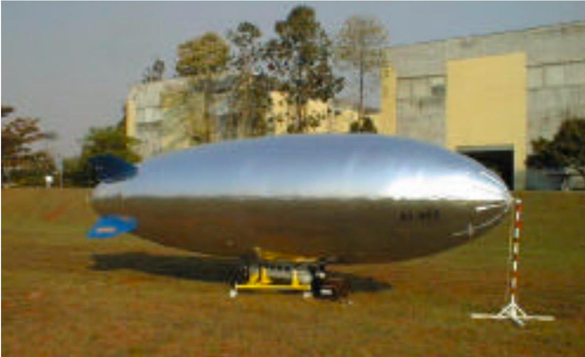
AURORA I airship is a modified Airspeed Airships AS-800. Source: Josué Ramos, et al. (2001)
