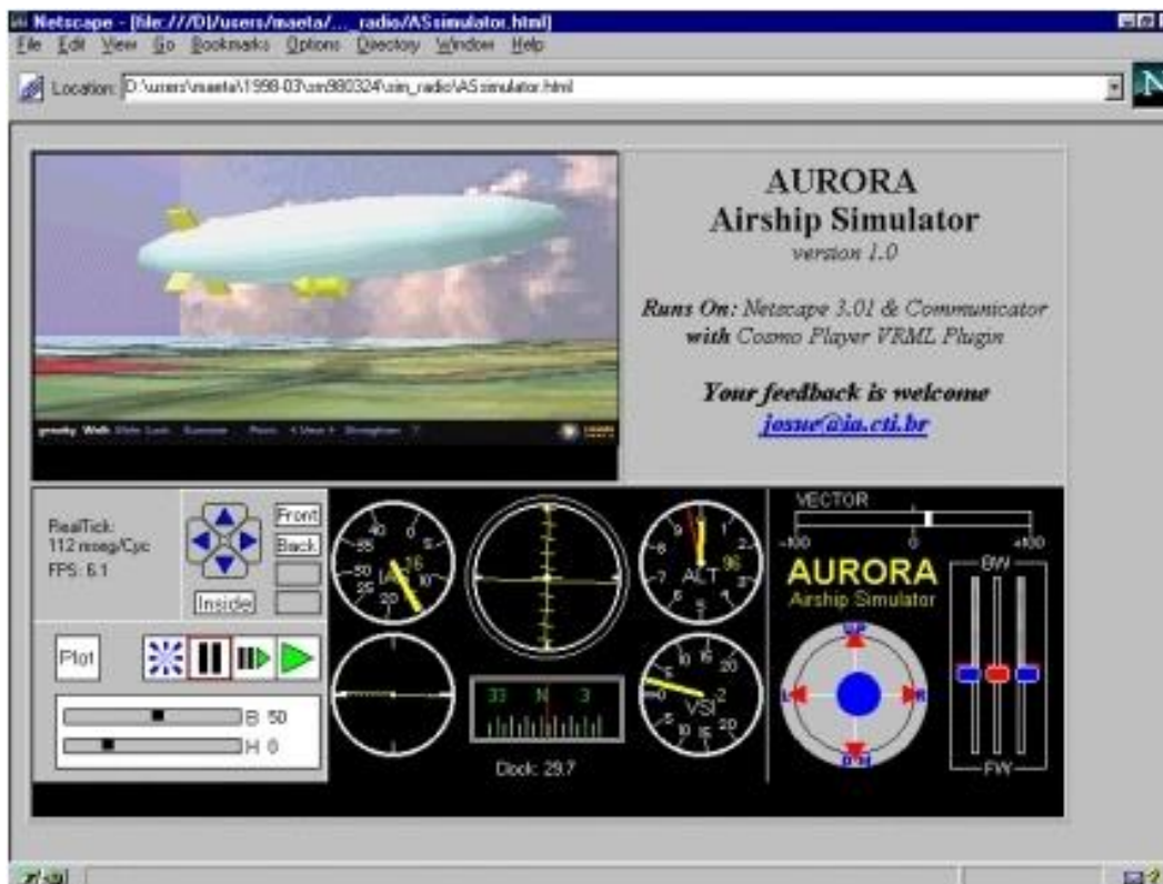
AURORA I flight simulator & virtual cockpit instruments. Source: Alberto Elfes, et al. (1998)
