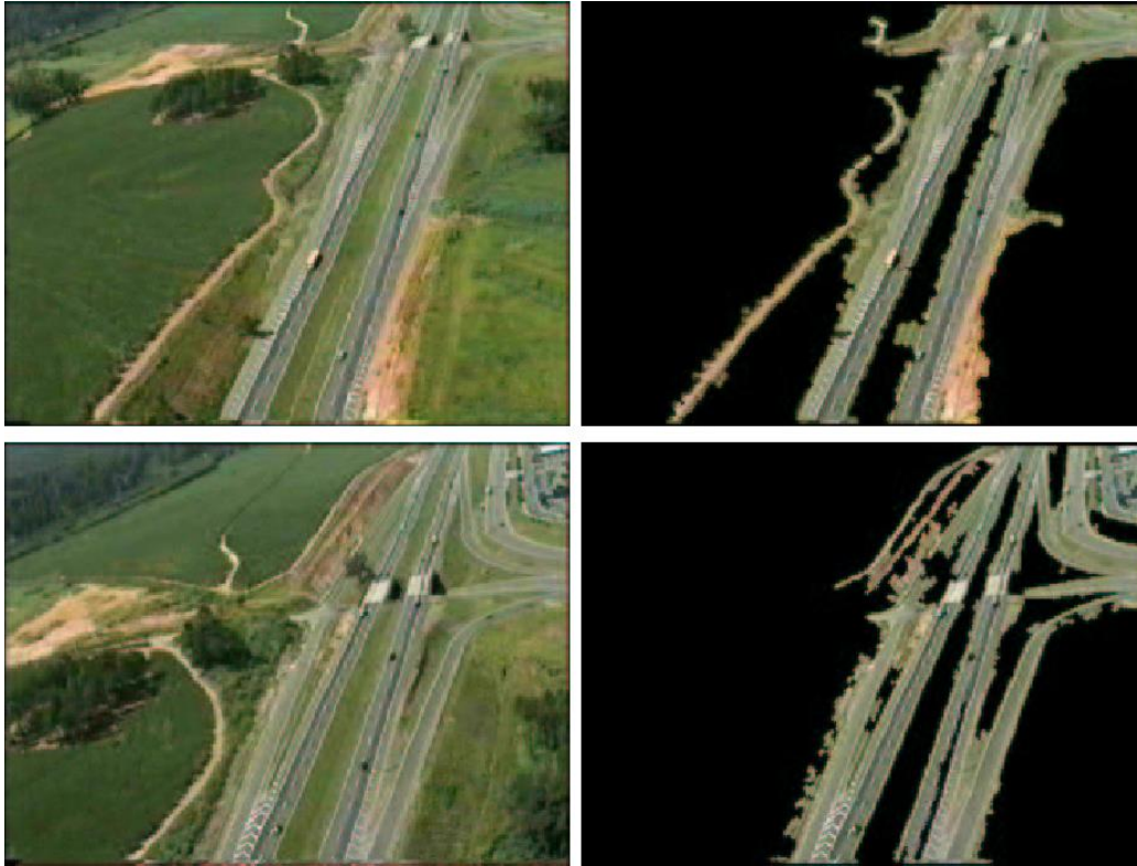
Identification and tracking of a paved road using an airborne camera. The aerial imagery is shown on the left, and the results of the target classification procedure on the right. Source: Bueno, et al., (2002)
