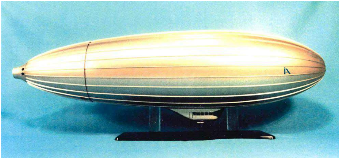
MC-7 model, exterior arrangement. The annular air inlet for the internal contra-rotating propellers is the vertical stripe (left of center). The main propulsion exhaust nozzle is visible at the stern. Source: Deans' Garage
