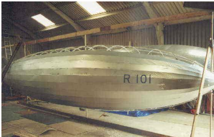
R101 model under construction at Airspeed Airships, showing rigid hull framework. Source, both photos: AHT
