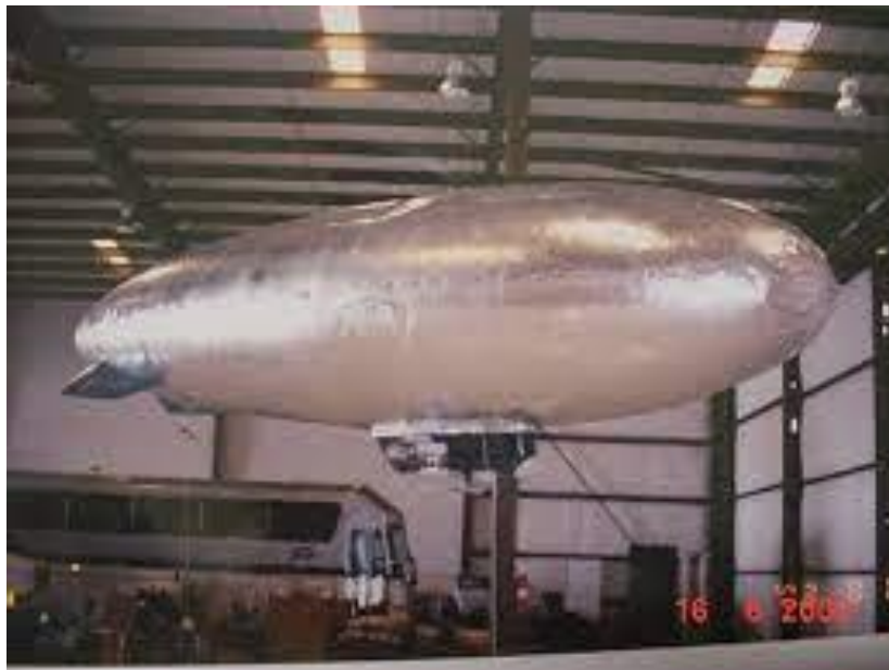
Indoor flight test of Gibbens' Airspeed blimp adapted for cycloidal propeller testing. Note that the upper tail fins have been removed. Source: Roy P. Gibbens (photo 2001)
