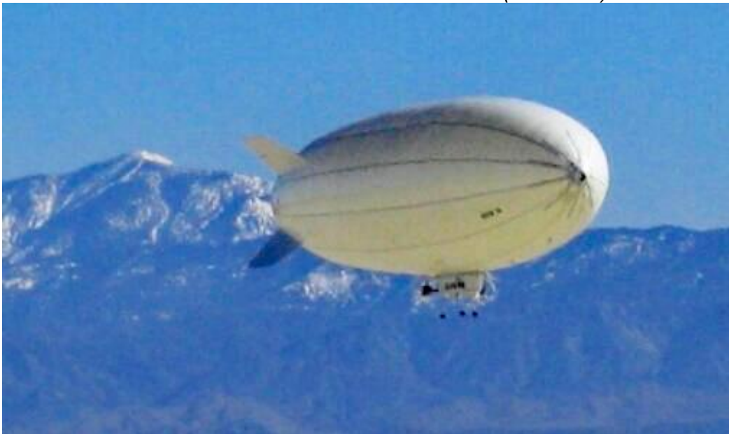
Autonomous flight of the JPL aerobot, conducted at the El Mirage dry lake in the Mojave desert. Source, both photos: JPL (Oct 2006)
