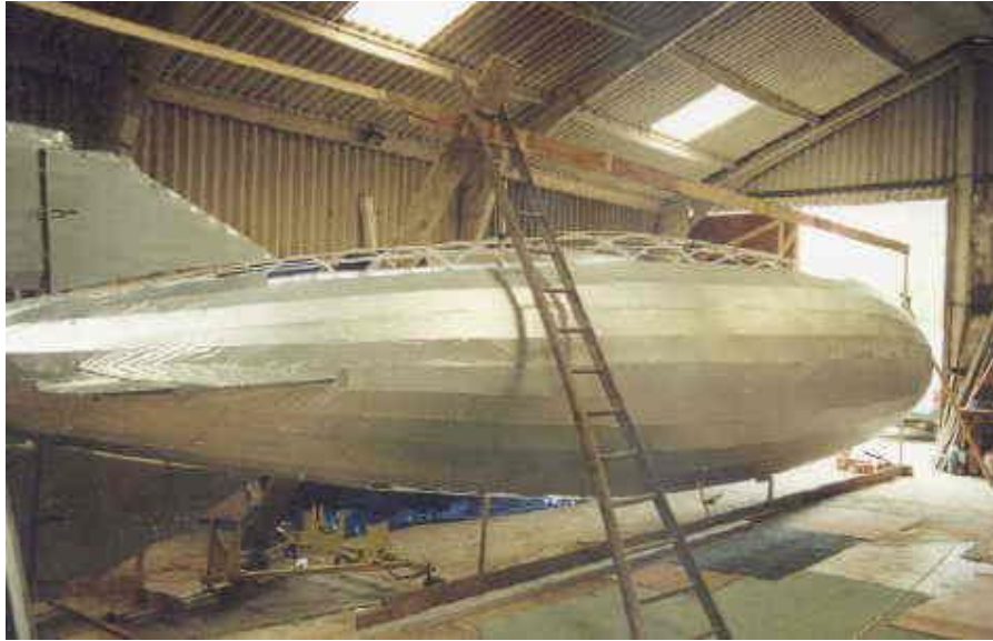
R101 model under construction showing rigid hull framework.
