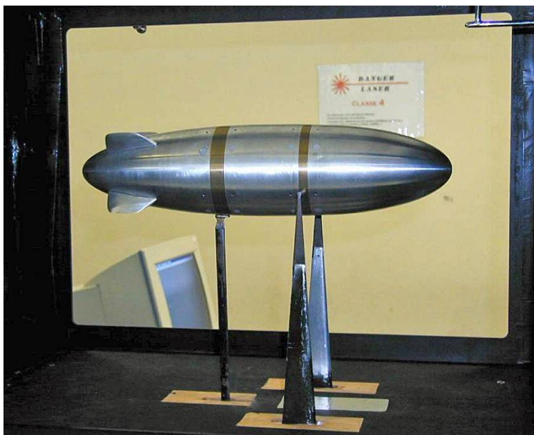
Scale wind tunnel model of the Karma V1 AS-500 was used to determine aerodynamic parameters later used in airship dynamic control models. L. Solaque & S.Lacroix, "Airship control" (2007)
