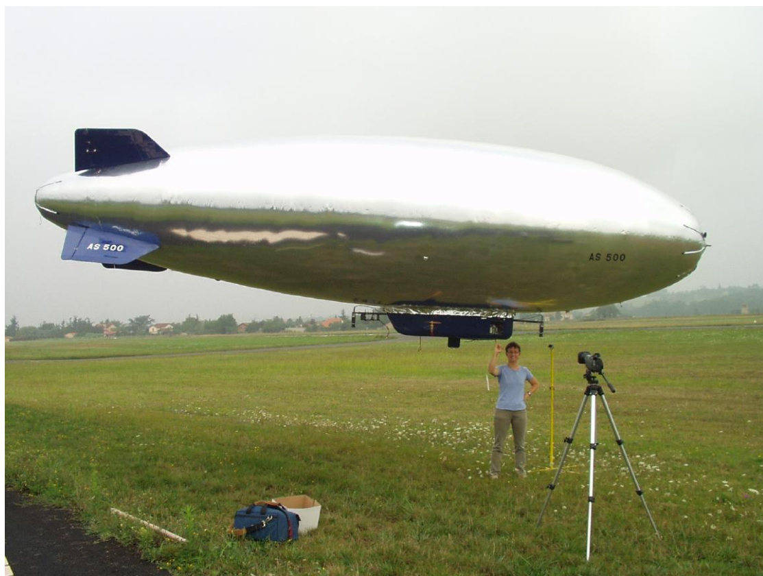
Karma V1 ready for fifth flight, with stern thruster removed (August 2002). Source, both photos: LAAS
