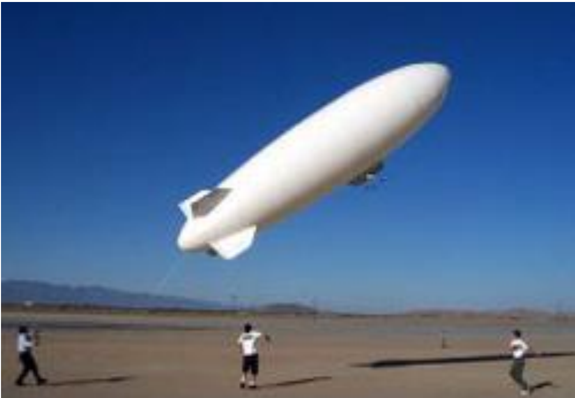
Takeoff of JPL's AS-800B aerobot, conducted at the El Mirage dry lake in the Mojave desert. Source, both photos: JPL
