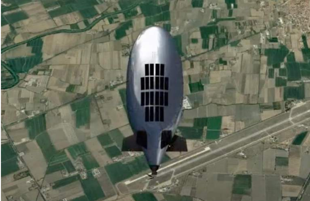
HHAA rotates to horizontal attitude after full inflation.
