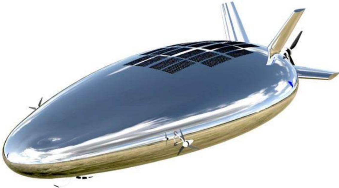
CIRA High Altitude Hybrid Airship (HHAA). Source: CIRA (2017)
