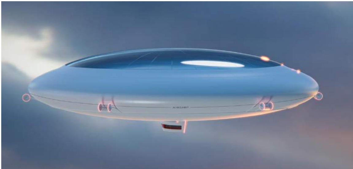
Lenticular airship showing placement of the horizontal axis cycloidal propellers around the periphery of the hull. Source: Juliana Juleva via Behance
