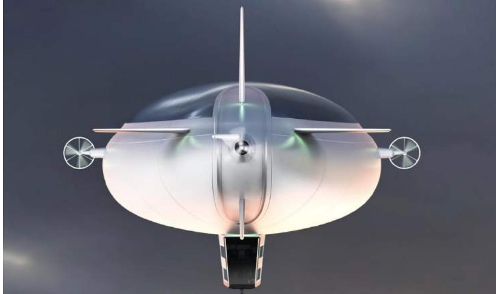
Views from behind the airship showing the placement of the flank-mounted main propellers and the tail-mounted longitudinal and lateral propellers.
