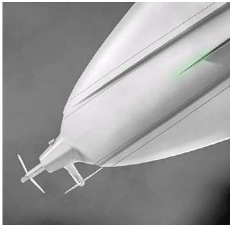
Closeup views of the longitudinal & lateral thrust propellers.
