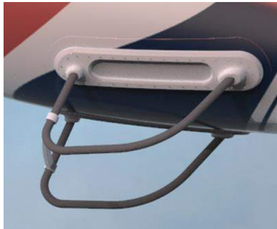
On the ground, the airship sits on two fixed landing skids forward and the two lower tail fins aft.
