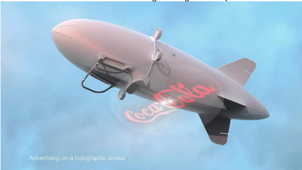
Rendering showing a concept for advertising displayed using a rotating holographic fan projector under the AirOne blimp. Source, both graphics: Juliana Juleva via Behance
