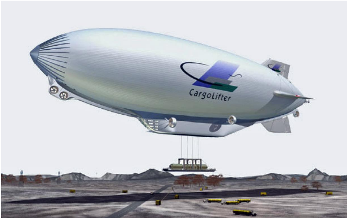
CL160 hovering with the loading frame partially lowered and secured to the ground by four cables. Source: CargoLifter
