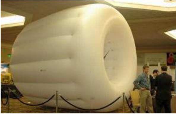
Cylindrical aerostat with wind turbine installed Source: RadioLocman (30 April 2011)
