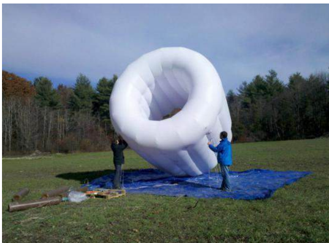
Hollow cylindrical aerostat test, November 2010. Sources: (L) RadioLocman (30 April 2011), (R) Altaeros
