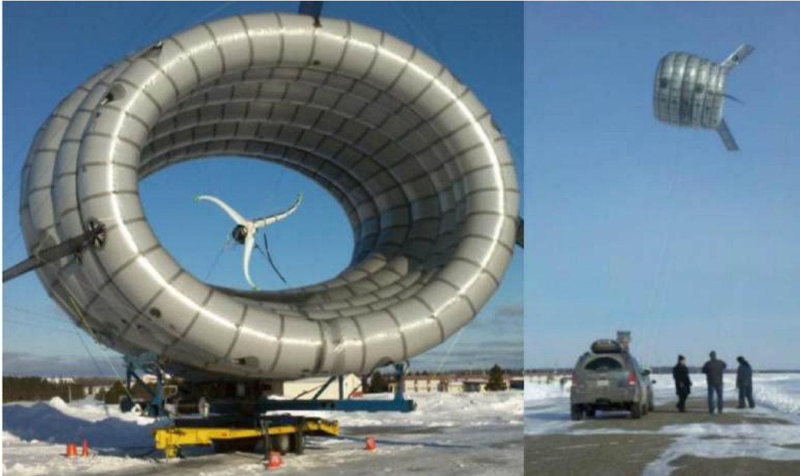
The proof-of-concept BAT tested at Loring AFB, Maine in 2012. Source: Altaeros (filing with Alaska Energy Authority, 2012)
