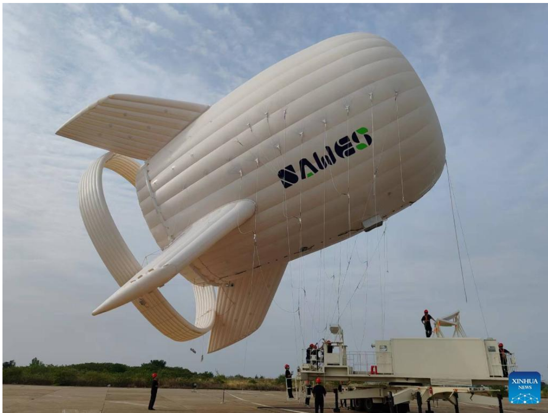
Tethered S500 buoyant airborne turbine (BAT) and its base station. Source: China Daily (photo taken 10 Oct 2024)
