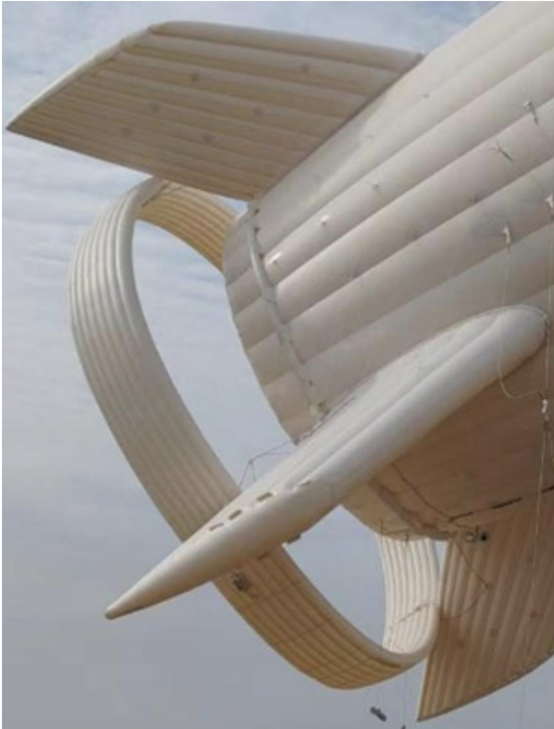
Closeup view of the ring tail configuration on the tethered S500 BAT. Source: China Daily (photo taken 10 Oct 2024)
