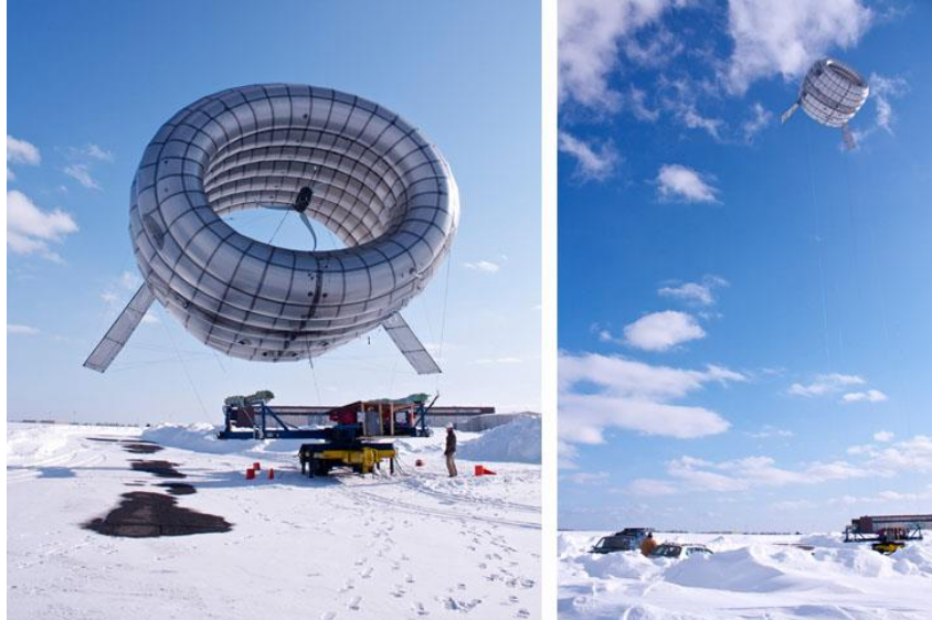
Altaeros BAT operational testing. Source: Altaeros (circa 2012)
