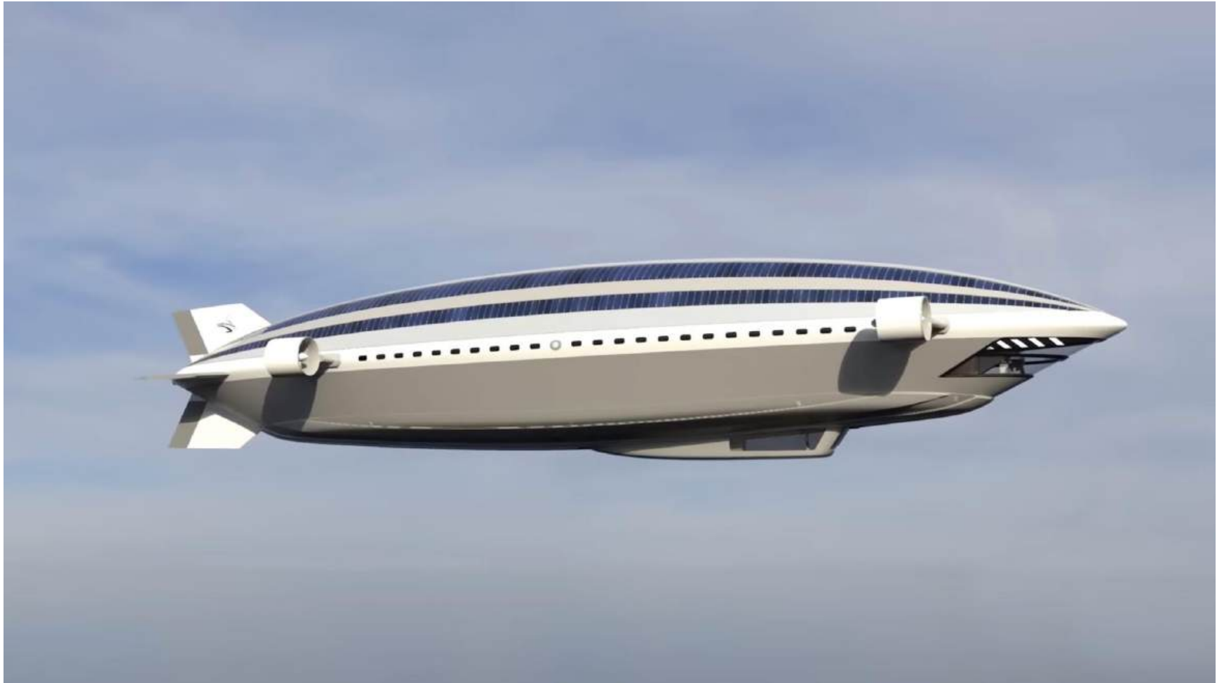
Norge 2.0 side view in cruise flight with the shrouded propulsors rotated to the horizontal position. The crew and passengers enter the airship via the small gondola under the hull. Source: Lazzarini
