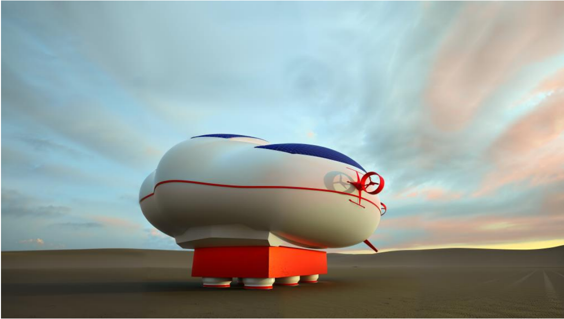
Bow quarter view of an Air Cube on the ground, sitting on its ACLS pads.
