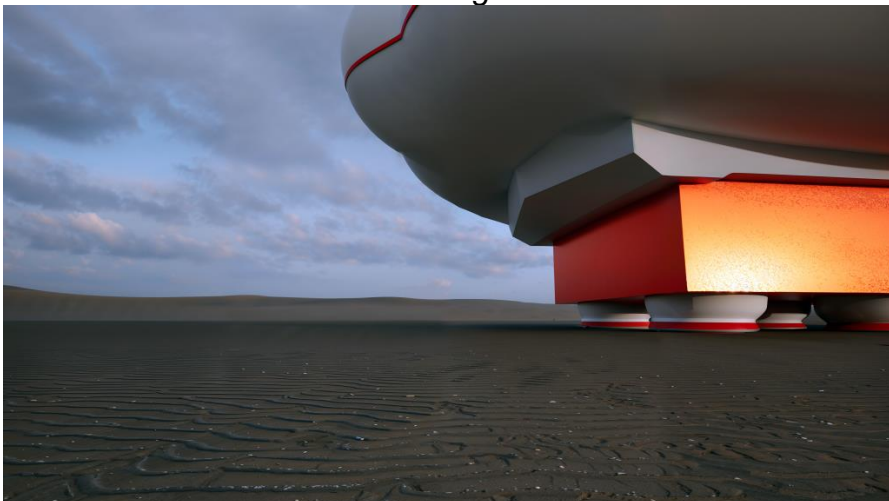
Stern quarter view showing the interface between the hybrid airship and the "Red Box" module containing the Sky Yacht's passenger accommodations. Source, three graphics: LDWO.
