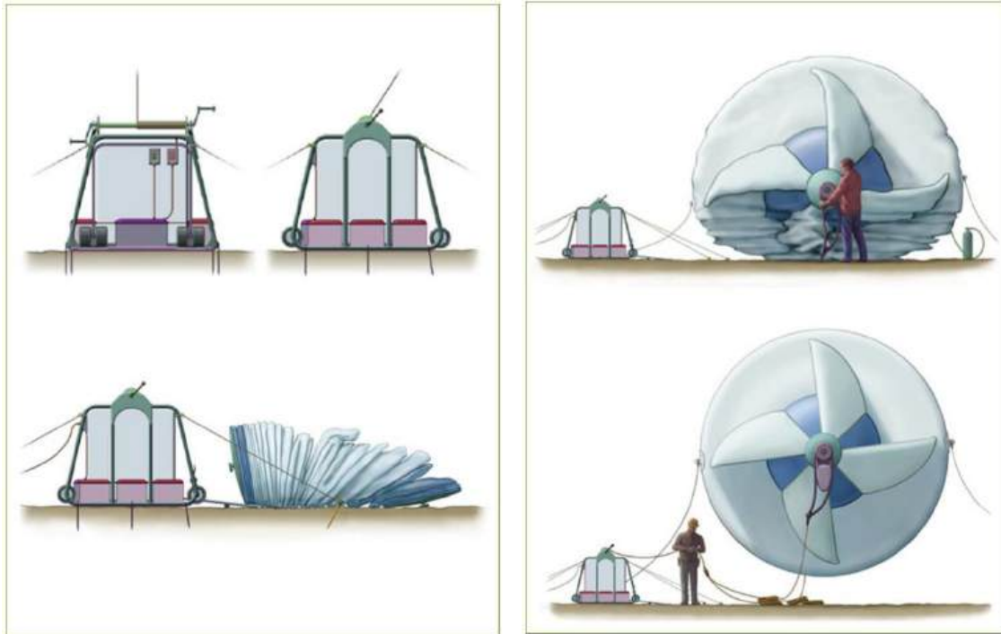
Deploying a small MARS unit (smaller than a 10 kW MARS). Source: Chris Radisch via Magenn Power
