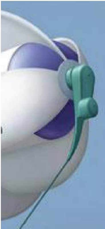
(L) Generator casing, yoke & tether (all green) connected to axle at one end of a 10 kW MARS airborne rotor.
