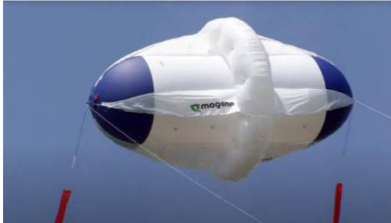
Early Magenn small-scale buoyant prototype with an inflated wind vane stabilizer, no generator, circa mid-2006.
