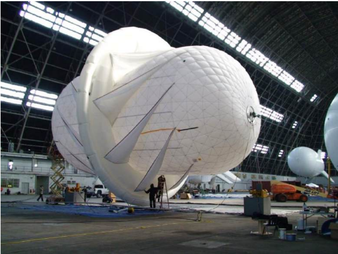
Fully-inflated Alpha prototype sitting on its wind vane stabilizer. Source: Magenn Power via screenshot from video
