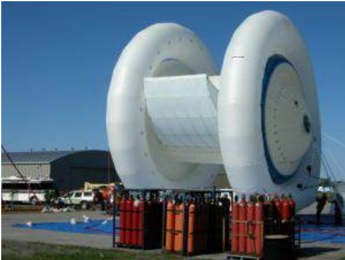
100 kW MARS secured on the ground. Source: Magenn Power via Design Engineering (2009)
